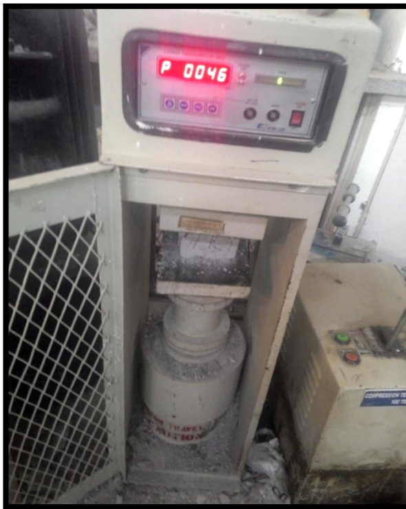
Fig.3.5 Universal Testing machine (UTM) Fig.3.6 Cube after compression failure
