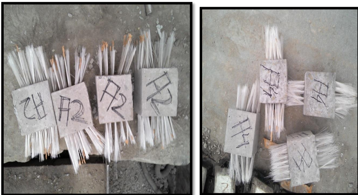
Fig.3.15 Cubes after unmoulding
