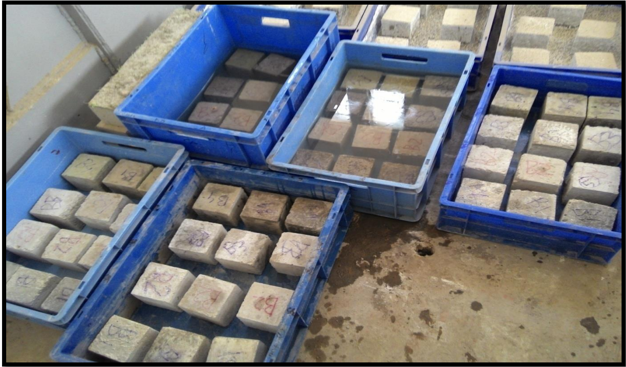
Fig.3.22 Placing of cube specimen in sulphuric acid and sodium sulphate solution
