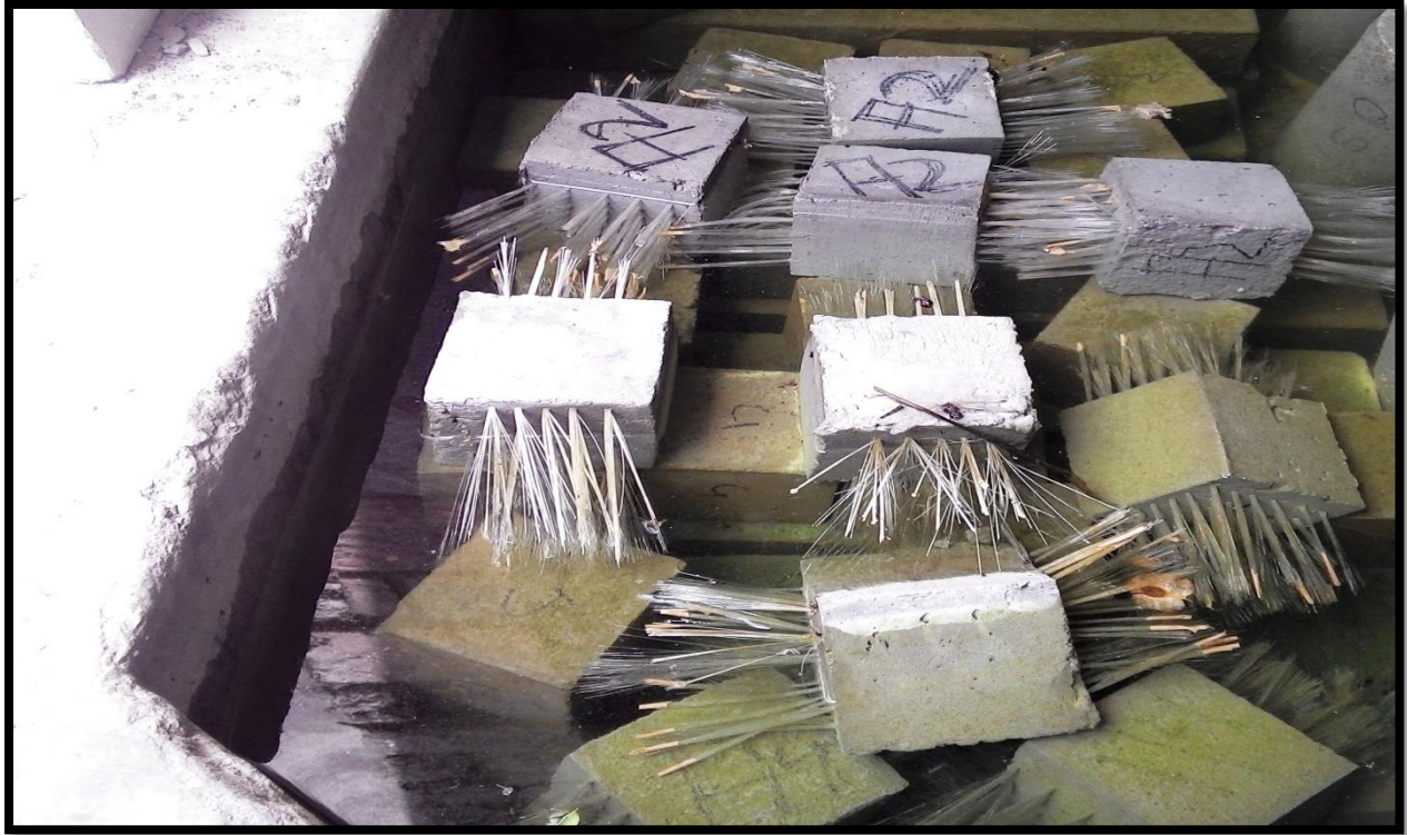
Fig.3.16 Curing of cubes
