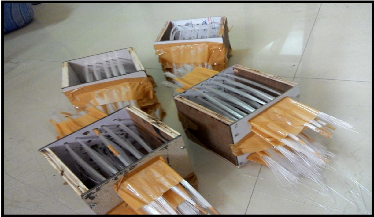
Fig.3.13 Placing of fibers in the mould
