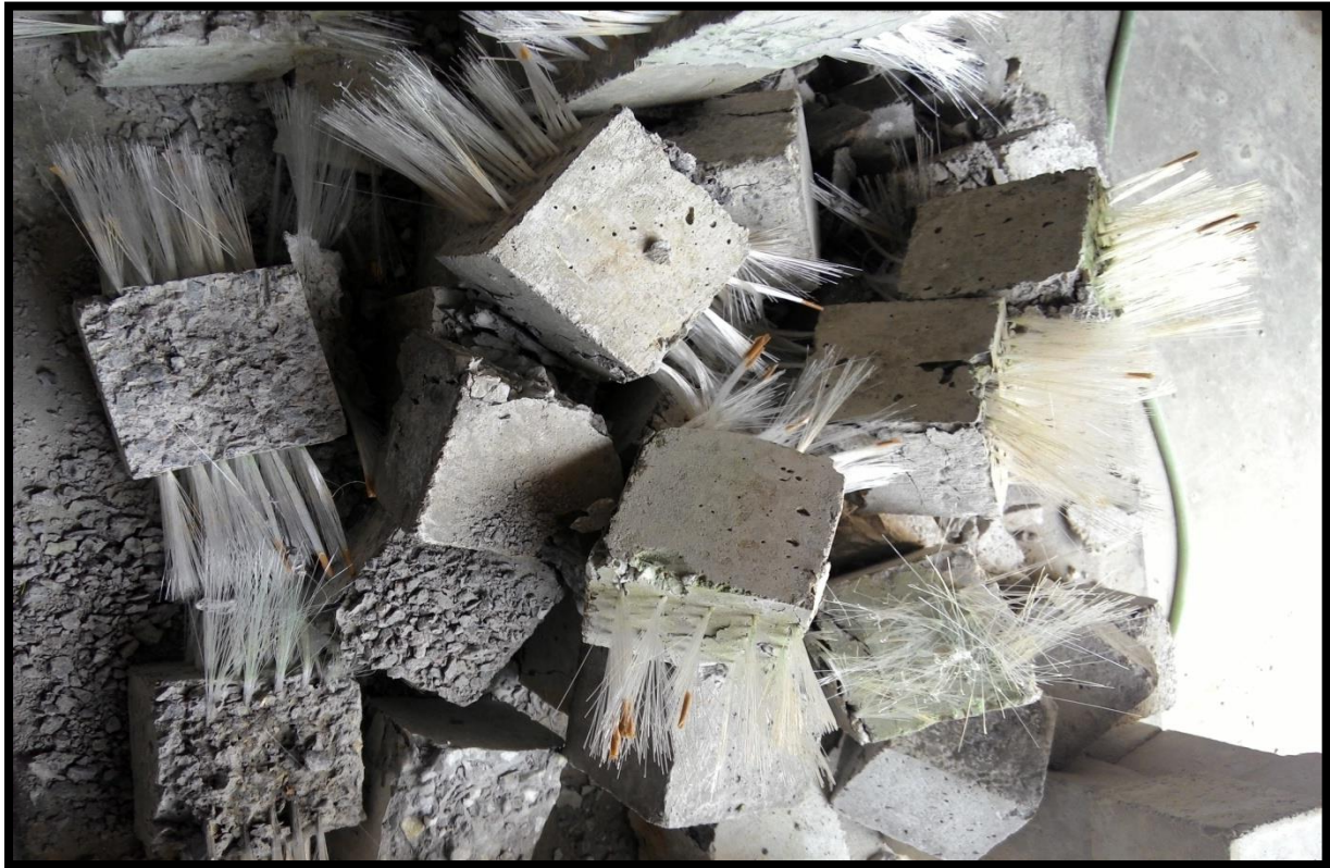
Fig.3.21 Light transmitting cubes after failure
