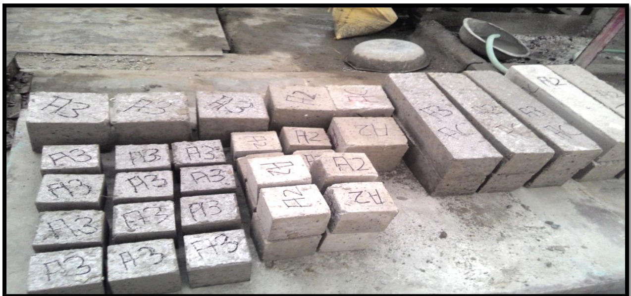
Fig.3.4 Casting of cube and beam specimen
