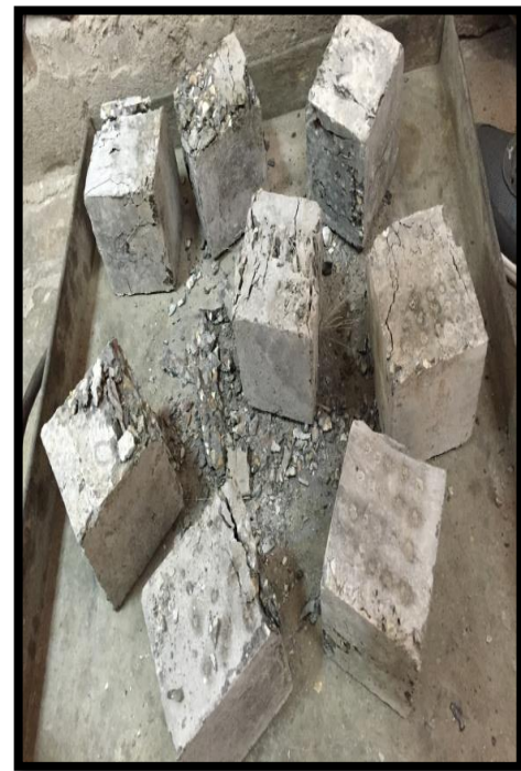
Fig.3.5 Universal Testing machine (UTM) Fig.3.6 Cube after compression failure
