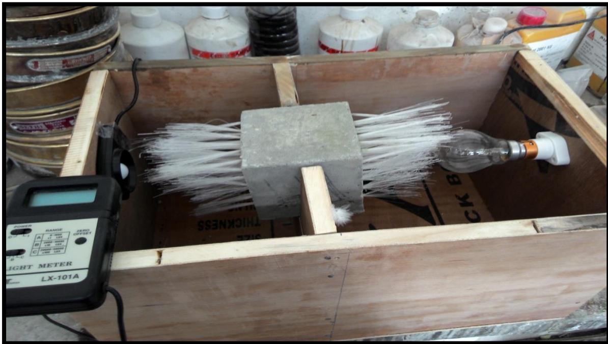
Fig.3.18 Experimental setup of light transmitting concrete
