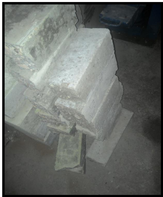
Fig.3.8 Beam after failure
