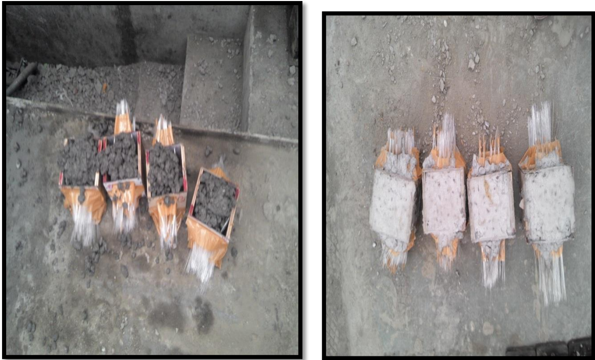
Fig.3.14 Casting of light transmitting cube
