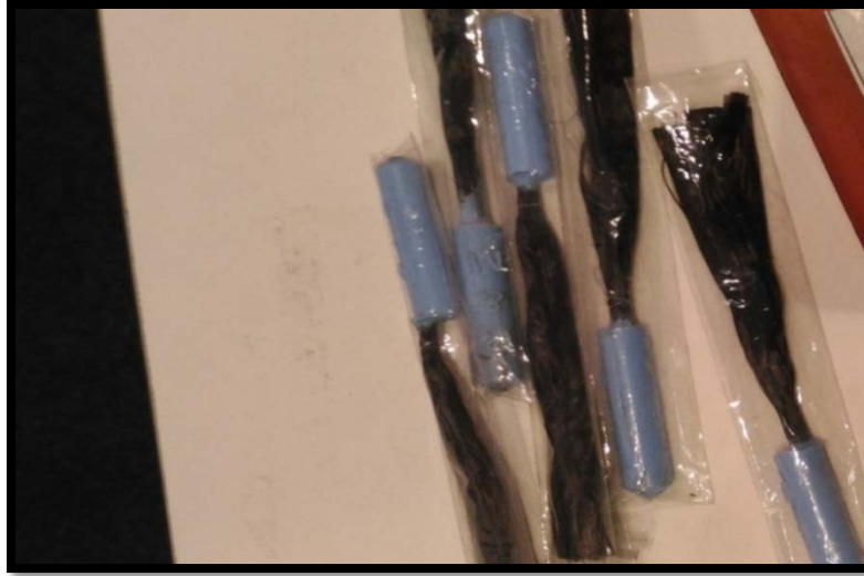
Figure.2.19:-Fiber used for Lapping of FRP wrapping.
