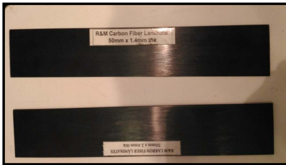
Figure 1.1:-Typical FRP Laminate
