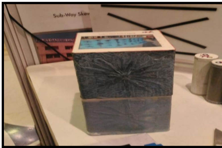
Figure.2.20:-Fiber used for Lapping of FRP wrap.
