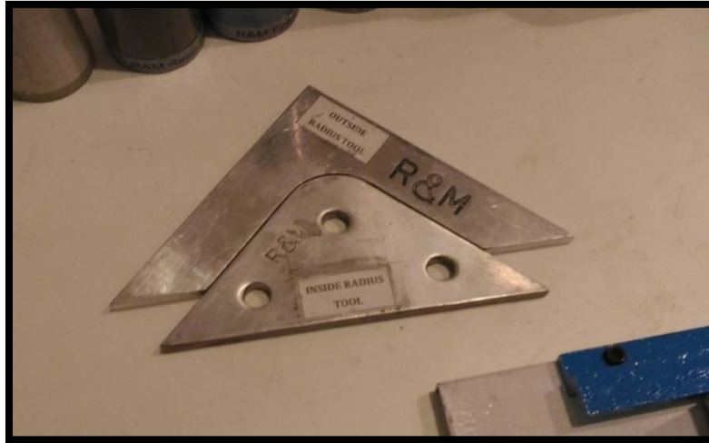
Figure.2.18:-Equipment used for chamfering column edge.
