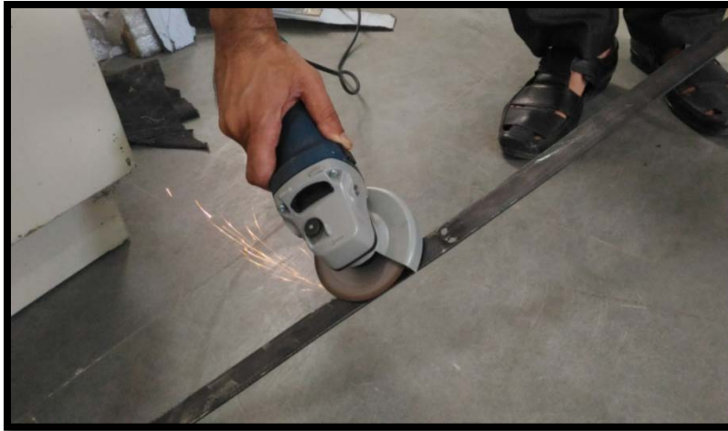
Figure.2.11:-Removing Oil Film Steel Plate.
