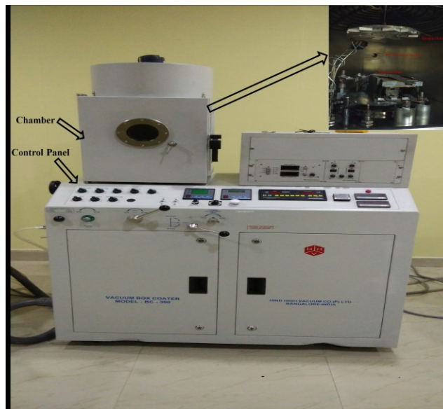
Figure 3.2 Thermal Vapor Deposition Machine
