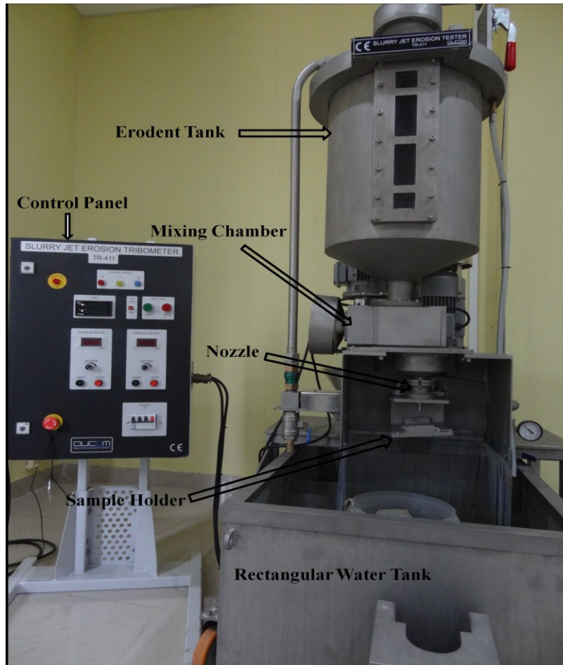
Figure 3.10 Slurry Jet Erosion Tester
