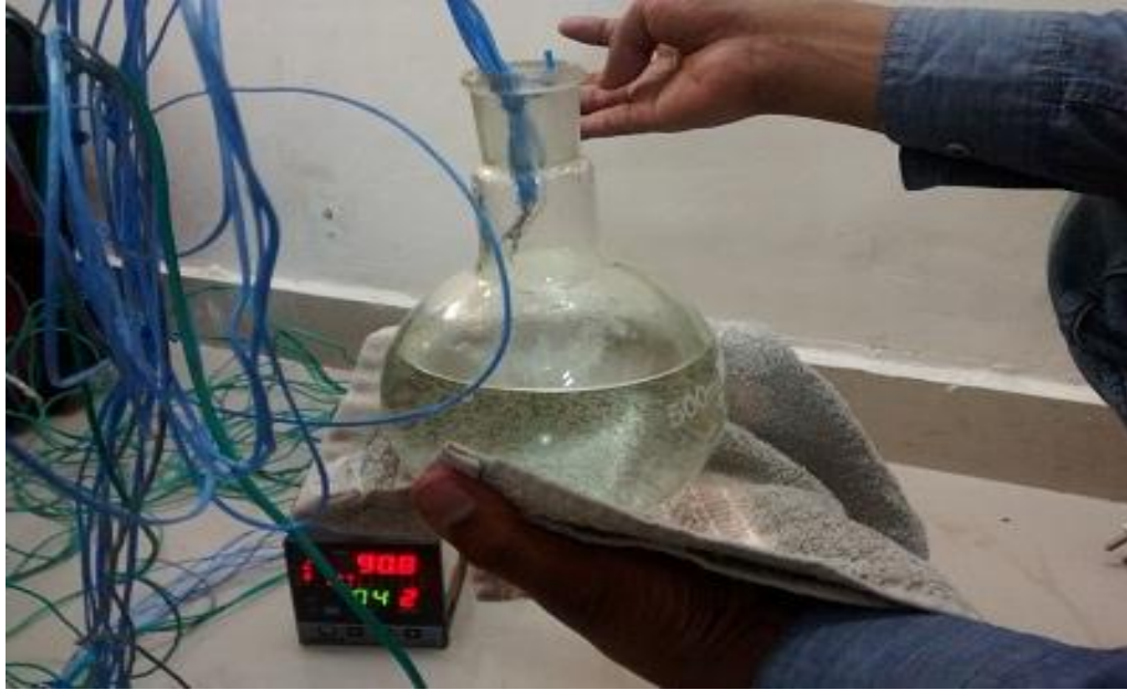
Figure: 4.5 Thermocouples calibration
