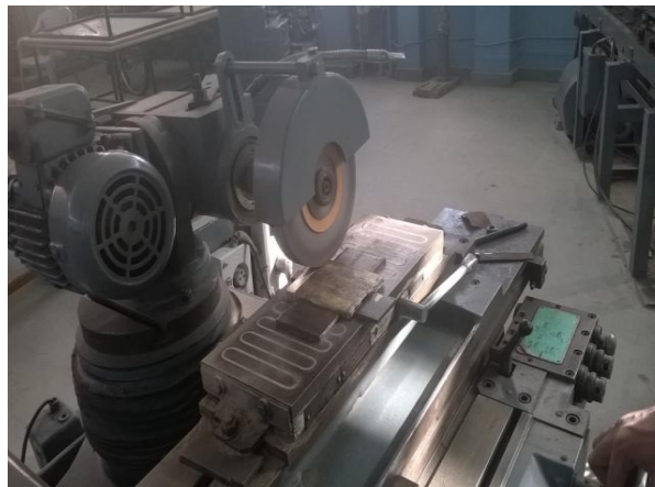
Figure 11: Surface grinding operation
