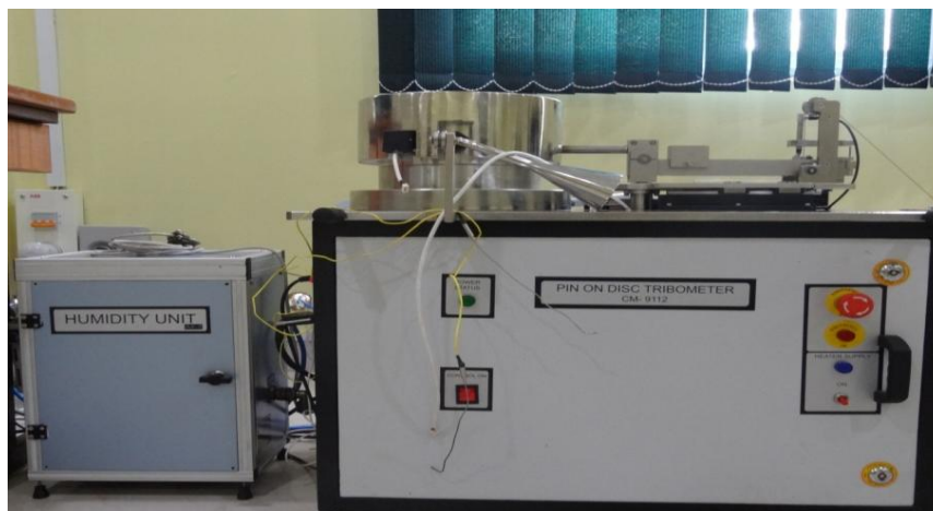
Figure 20: Figure Equipment used to perform sliding wear test (pin on discTribometre)
