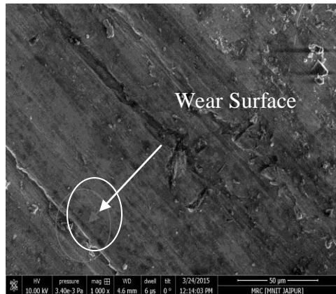
Figure 41: SEM images of 4 wt% dual reinforcement
