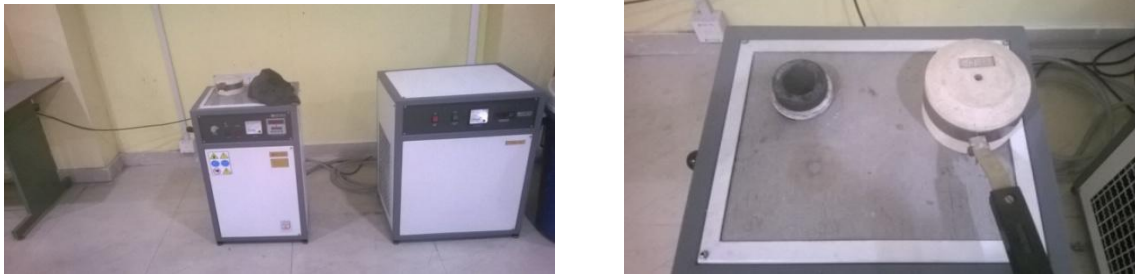
Figure 10: Furnance for preheating the reinforcement
