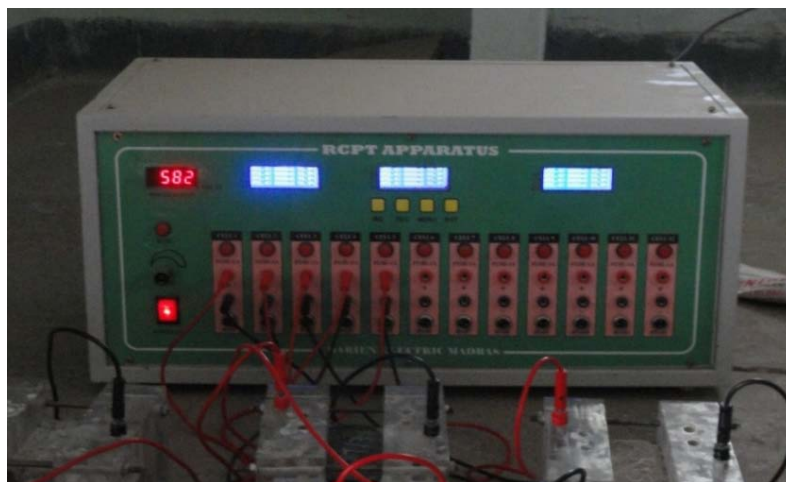
Fig. 4.5 Chloride penetration measurement apparatus
