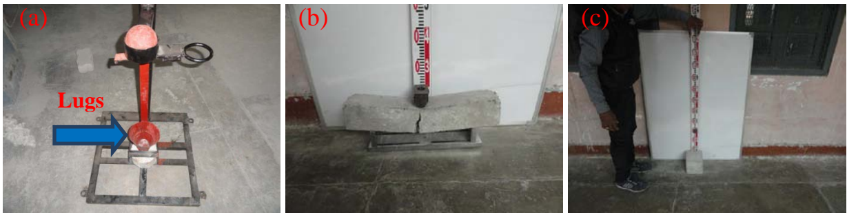
Fig. 5.3 (a) Drop weight test; (b) Flexural test; and (c) Rebound test
