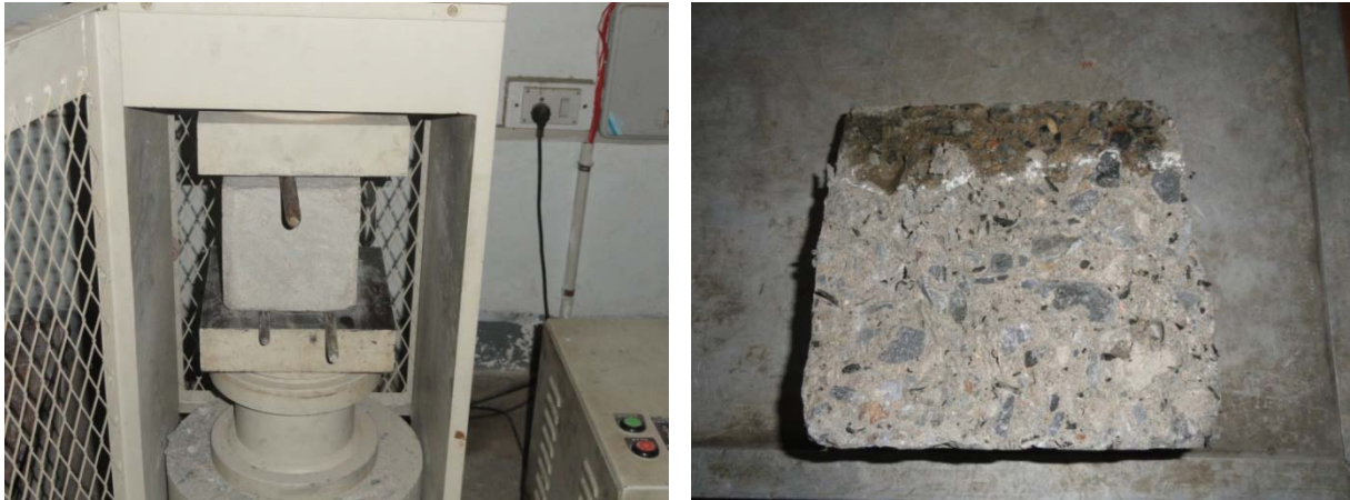
Fig. 4.2 Arrangement for splitting cubes for measurement of water permeability depth
