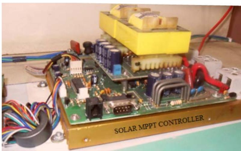
Figure 5.2 Hardware configuration of solar MPPT controller
