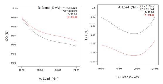
Fig. 4.30 Variation in CO with load and n-butanol-diesel blends at minimum and maximum values
