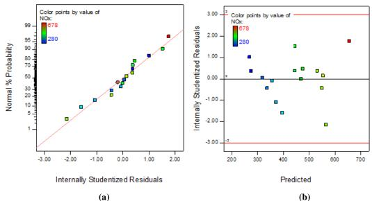
Fig. 4.8 (a) Plot of normal % probability vs. internal studentized residuals for NO<sub>x</sub>
