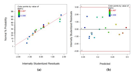
Fig. 4.73 (a) Plot of normal % probability vs. internal studentized residuals for BSFC(b) Plot of internal studentized residuals vs. predicted response for BSFC
