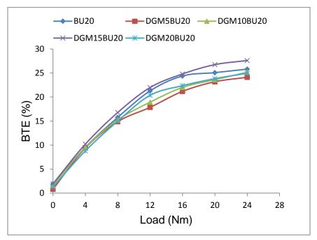
Fig. 4.83 Variation of BTE with engine load for Diglyme-BU20 blends
