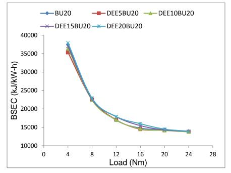
Fig. 4.102 (b) Variation of BSEC with engine load for Diethylether-BU20 blends
