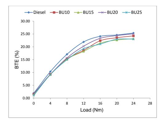
Fig. 4.18 Variation of BTE with engine load for diesel and n-butanol-diesel blends
