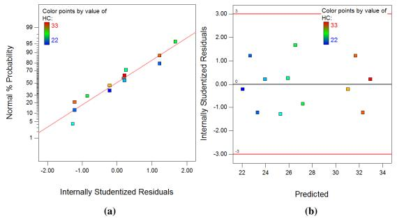
Fig.4.57 (a) Plot of normal % probability vs. internal studentized residuals for HC(b) Plot of internal studentized residuals vs. predicted response for HC
