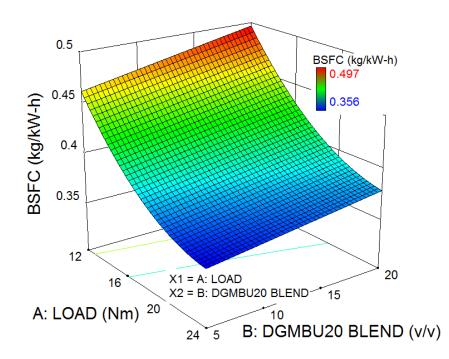
Fig. 4.82 Variation in BSFC due to combined effect of load and Diglyme blending
