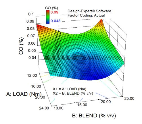
Fig. 4.29 Variation in CO due to combined effect of load and n-butanol blending
