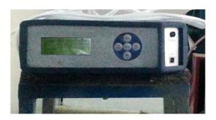
Fig: 3.4 AVL Exhaust gas analyzer
