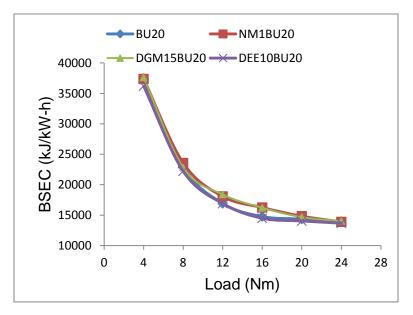
Fig. 4.116 (b) Variation of BSEC with engine load for different blended fuels
