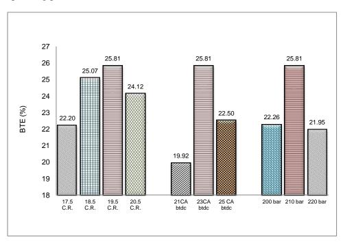
Fig. 4.42 BTE at different CRs, injection timings and injection pressures for BU20
