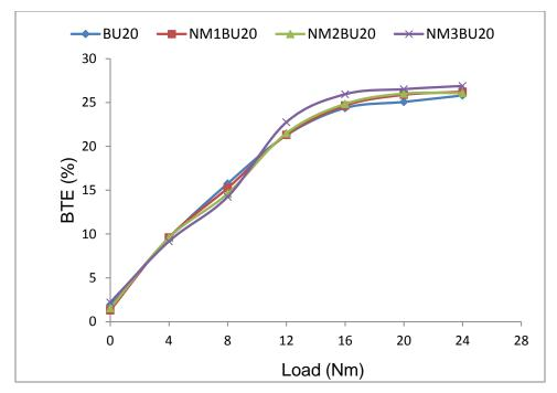
Fig. 4.62 Variation of BTE with engine load for NM-BU20 blends
