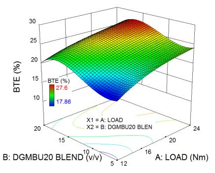
Fig. 4.84 Variation in BTE due to combined effect of load and Diglyme blending
