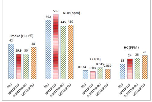
Fig. 4.123 Comparison of smoke, NO<sub>x</sub>, HC and CO at full load for different blended fuels<sup>4</sup>
