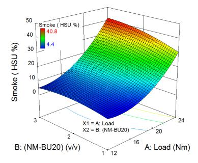
Fig. 4.65Variation in smoke due to combined effect of load and NM blending
