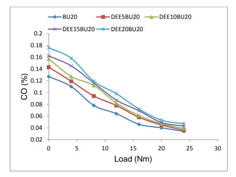
Fig. 4.110 Variation in CO for Diethylether-BU20 blends
