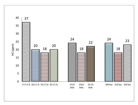
Fig. 4.50 HC emission at different CRs, injection timings and injection pressuresfor BU20
