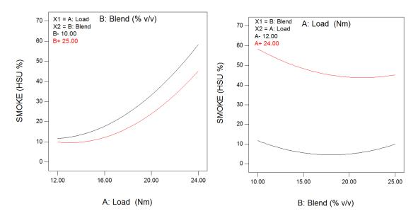
Fig. 4.23 Variation in smoke with load and n-butanol-diesel blends at minimum and maximum values
