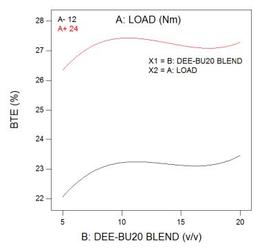
Fig. 4.105 Variation in BTE with diethylether blending at medium and full load
