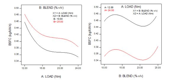
Fig. 4.15 Variation in BSFC with load and n-butanol-diesel blends at minimum and maximum values
