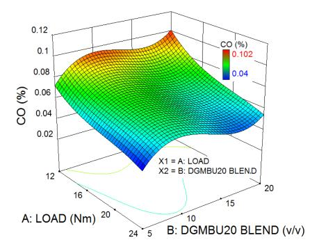
Fig. 4.90 Variation in CO due to combined effect of load and Diglyme blending
