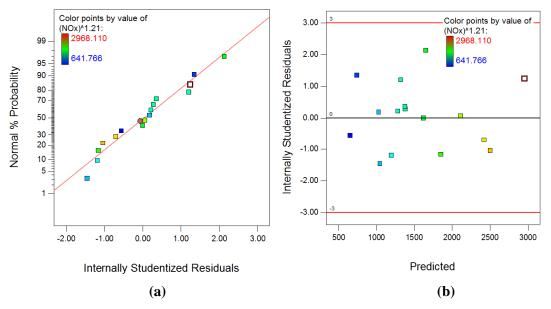
Fig. 4.97 (a) Plot of normal % probability vs. internal studentized residuals for NO<sub>x</sub>
