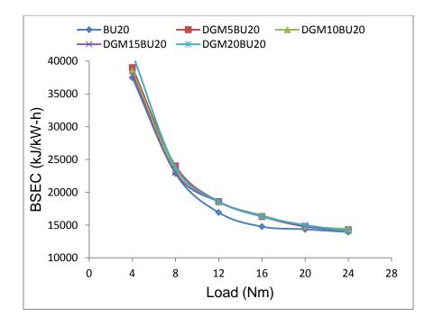
Fig. 4.81(b) Variation of BSEC with engine load for Diglyme-BU20 blends
