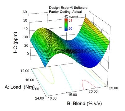
Fig. 4.32 Variation in HC due to combined effect of load and n-butanol blending
