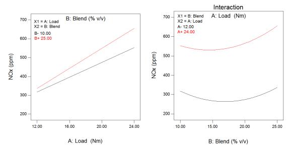
Fig. 4.26 Variation in  $NO_x$  with load and n-butanol-diesel blends at minimum and maximum values
