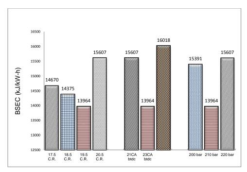
Fig. 4.41 (b) BSEC at different CRs, injection timings and injection pressures for BU20
