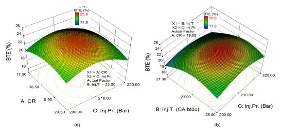
Fig. 4.43 Variation in BTE due to combined effect of (a) CR and injection pressure and (b) injection timing and injection pressure for BU20
