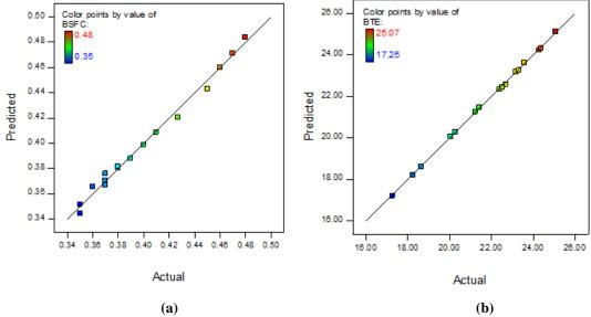
Fig. 4.11 Plot of actual values vs. predicted values for (a) BSFC (b)BTE
