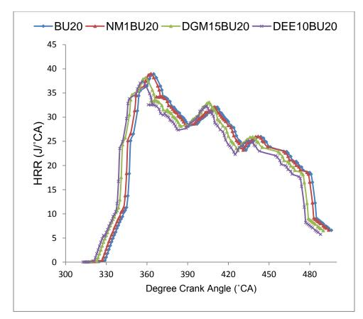
Fig. 4.115 Comparison of heat release rate of different blended fuels
