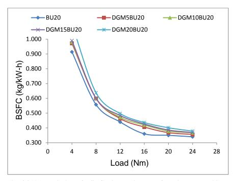
Fig. 4.81(a) Variation of BSFC with engine load for Diglyme-BU20 blends
