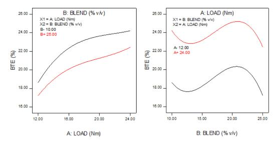
Fig. 4.20 Variation in BTE with load and n-butanol-diesel blends at minimum and maximum values
