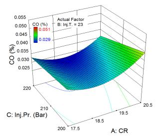
Fig.4.49 Variation in CO due to combined effect of CR and Injection Pressurefor BU20
