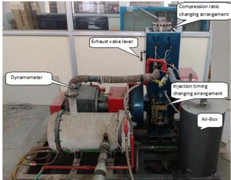
Fig. 3.2 Actual engine set-up
