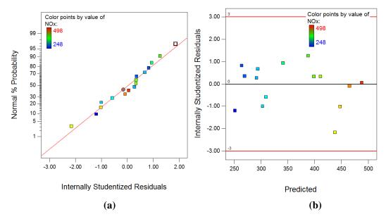
Fig. 4.76 (a) Plot of normal % probability vs. Internal studentized residuals for NO<sub>x</sub>
