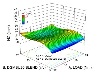
Fig. 4.92 Variation in HC due to combined effect of load and Diglyme blending
