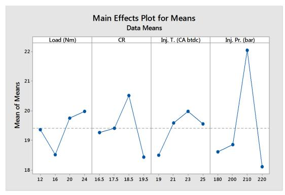
Fig. 4.2 Effect of engine operating parameters on BTE
