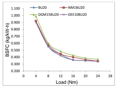
Fig. 4.116 (a) Variation of BSFC with engine load for different blended fuels
