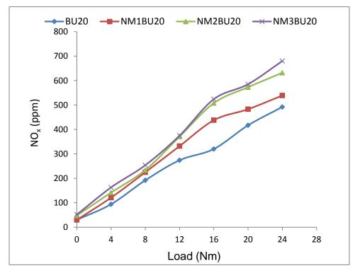
Fig. 4.66 Variation in NO<sub>x</sub> for NM-BU20 blends
