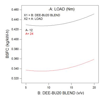
Fig. 4.103 Variation in BSFC with diethylether blending at medium and full load 4.7.3.2 Brake thermal efficiency
