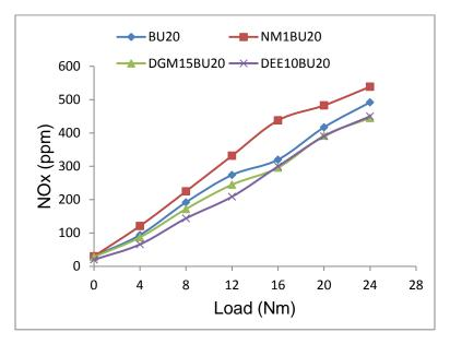
Fig. 4.119 Variation of NO<sub>x</sub> with engine load for different blended fuels
