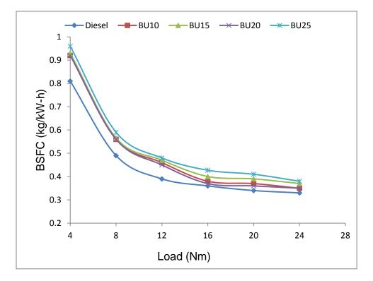
Fig. 4.13 Variation of BSFC with engine load for n-butanol-diesel blends
