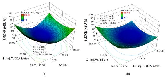
Fig. 4.45 Variation in smoke due to combined effect of (a) CR and injection timing and (b) injection pressure and injection timingfor BU20
