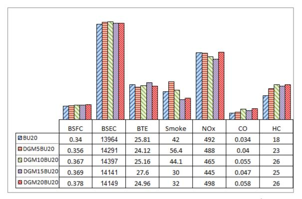
Fig. 4.93 Performance and emission of Diglyme-BU20 blends (100% rated power)<sup>2</sup>
