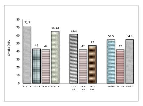
Fig. 4.44 Smoke emission at different CRs, injection timings and injection pressures for BU20
