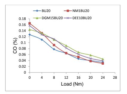
Fig. 4.120 Variation of CO with engine load for different blended fuels
