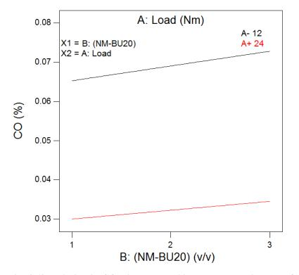
Fig. 4.69Variation in CO with NM-BU20 blends at medium and full load
