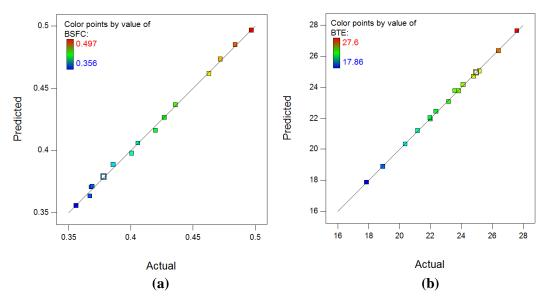
Fig. 4.79 Plot of actual values vs. predicted values for (a) BSFC (b) BTE
