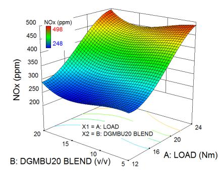
Fig. 4.88 Variation in NO<sub>x</sub> due to combined effect of load and Diglyme blending
