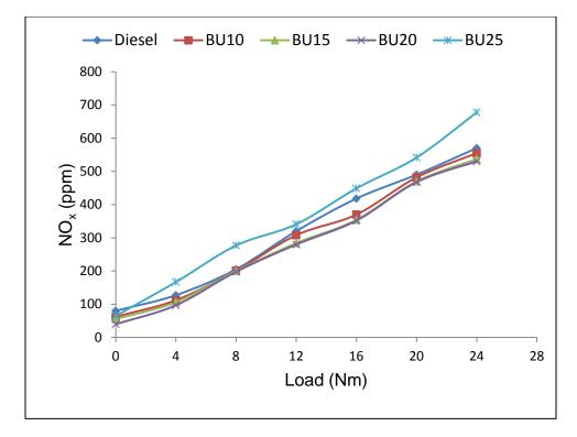
Fig. 4.24 Variation in NO<sub>x</sub> for n-butanol blends
