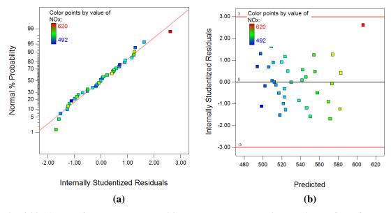
Fig. 4.38 (a) Plot of normal % probability vs. Internal studentized residuals for NO<sub>x</sub> (b) Plot of internal studentized residuals vs. predicted response for NO<sub>x</sub>
