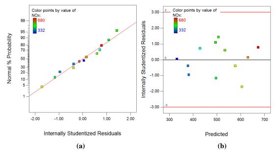
Fig. 4.55 (a) Plot of normal % probability vs. internal studentized residuals for NO<sub>x</sub>
