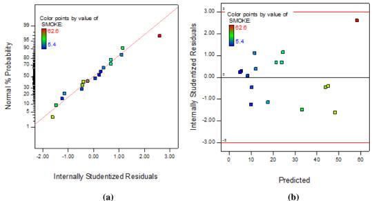
Fig. 4.7 (a) Plot of normal % probability vs. internal studentized residuals for smoke (b) Plot of internal studentized residuals vs. predicted response for smoke
