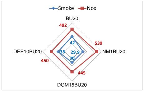
Fig. 4.124 Smoke-NO<sub>x</sub> Trade-off for different blended fuels
