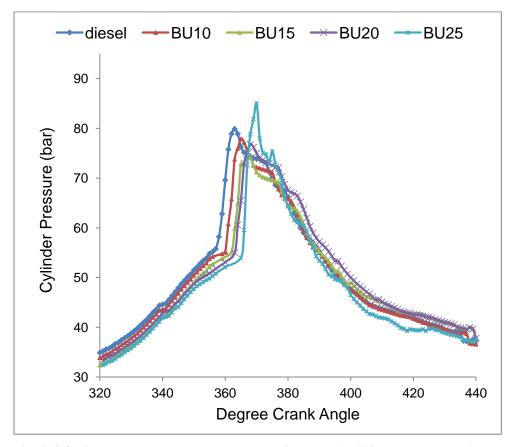
Fig. 4.4 Cylinder pressure vs. crank angle diagram (at 100% rated power)
