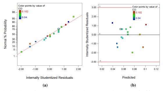
Fig. 4.77 (a) Plot of normal % probability vs. internal studentized residuals for CO (b) Plot of internal studentized residuals vs. predicted response for CO
