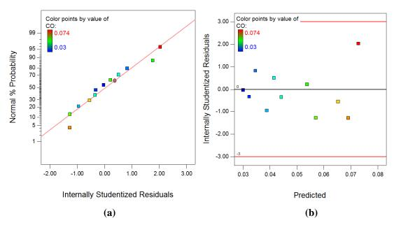
Fig. 4.56 (a) Plot of normal % probability vs. internal studentized residuals for CO (b) Plot of internal studentized residuals vs. predicted response for CO
