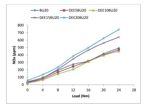
Fig. 4.108 Variation in NO<sub>x</sub> for Diethylether-BU20 blends
