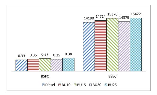
Fig. 4.17 Variation of BSFC and BSEC for different n-butanol-diesel blends at full load condition
