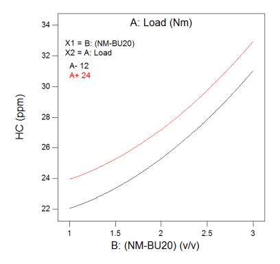
Fig. 4.71Variation in HC with NM-BU20 blends at medium and full load
