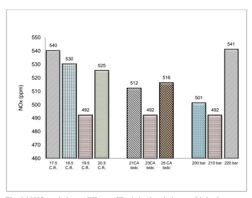
Fig. 4.46 NO<sub>x</sub> emission at different CRs, injection timings and injection pressures for BU20
