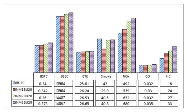
Fig. 4.72 Performance and emission of NM-BU20 blends (100% rated power)<sup>1</sup>
