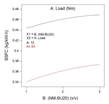
Fig. 4.61 Variation in BSFC with NM-BU20 blends at medium and full load
