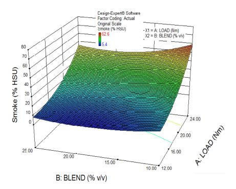
Fig. 4.22 Variation in smoke due to combined effect of load and n-butanol blending
