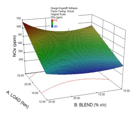
Fig. 4.25 Variation in NO<sub>x</sub> due to combined effect of load and n-butanol blending
