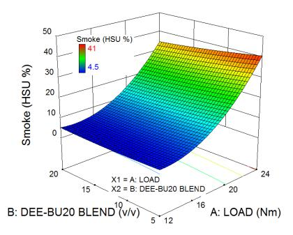
Fig. 4.107 Variation in smoke due to combined effect of load and Diethylether blending
