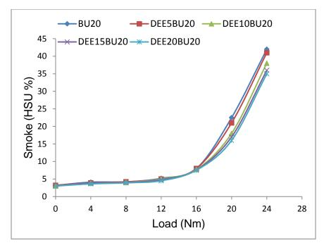
Fig. 4.106 Variation in smoke for Diethylether-BU20 blends
