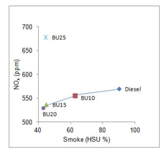
Fig. 4.27 Smoke-NO<sub>x</sub> trend for n-butanol diesel blends
