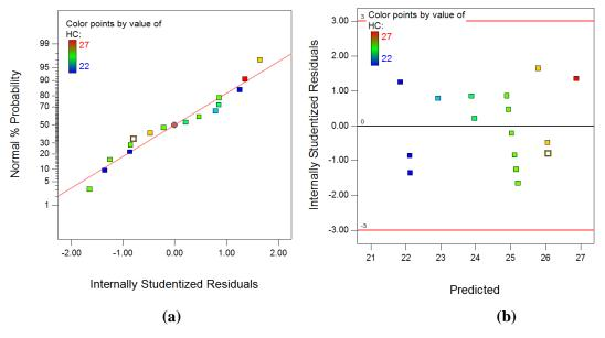
Fig.4.78 (a) Plot of normal % probability vs. internal studentized residuals for HC(b) Plot of internal studentized residuals vs. predicted response for HC
