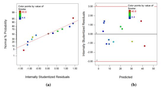
Fig. 4.54 (a) Plot of normal % probability vs. internal studentized residuals for smoke (b) Plot of internal studentized residuals vs. predicted response for smoke
