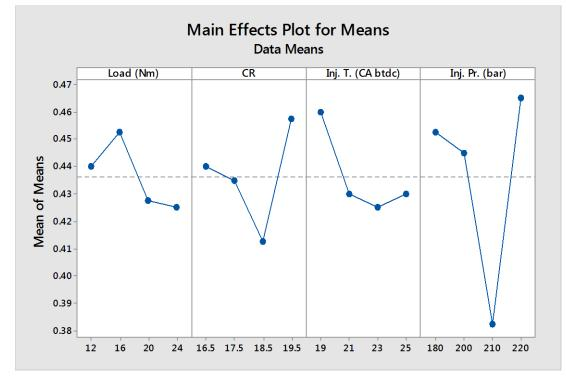
Fig. 4.1 Effect of engine operating parameters on BSFC
