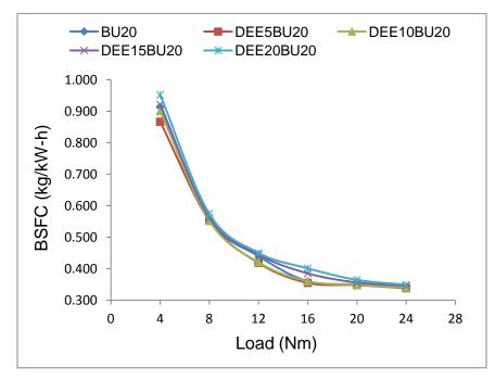
Fig. 4.102 (a) Variation of BSFC with engine load for Diethylether-BU20 blends
