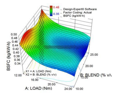
Fig. 4.14 Variation in BSFC due to combined effect of load and n-butanol blending
