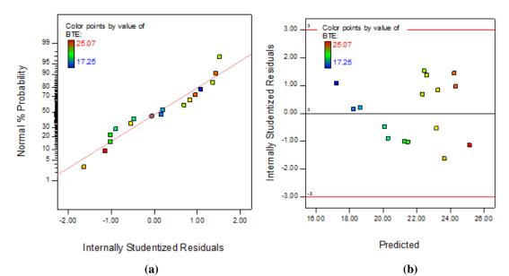
Fig. 4.6 (a) Plot of normal % probability vs. internal studentized residuals for BTE (b) Plot of internal studentized residuals vs. predicted response for BTE
