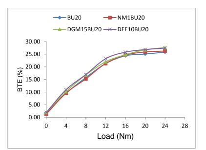
Fig. 4.117 Variation of BTE with engine load for different blended fuels
