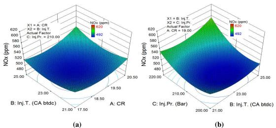
Fig.4.47 Variation in NO<sub>x</sub> due to combined effect of (a) CR and Injection Timing and (b) Injection Pressure and Injection Timingfor BU20
