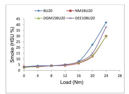
Fig. 4.118 Variation of smoke with engine load for different blended fuel
