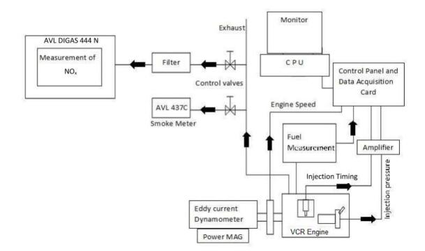
Fig. 3.1 (a) Schematic of engine set-up
