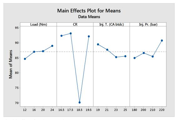
Fig. 4.3 Effect of engine operating parameters on smoke
