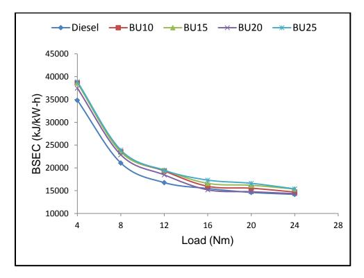
Fig. 4.16 Variation of BSEC with engine load for n-butanol-diesel blends
