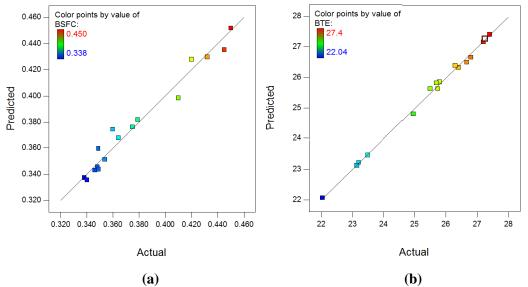
Fig. 4.100 Plot of actual values vs. predicted values for (a) BSFC (b)BTE
