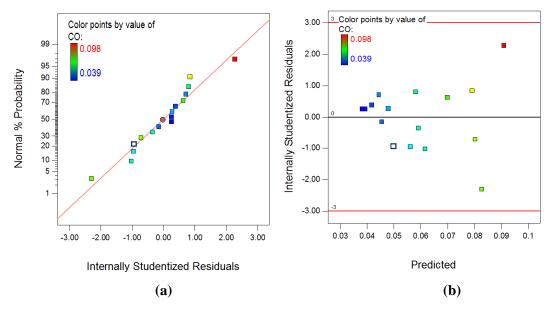
Fig. 4.98 (a) Plot of normal % probability vs. internal studentized residuals for CO (b) Plot of internal studentized residuals vs. predicted response for CO
