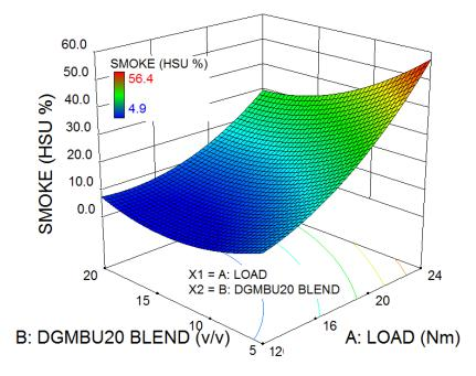
Fig. 4.86 Variation in smoke due to combined effect of load and Diglyme blending
