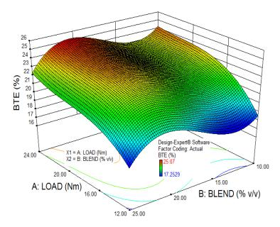
Fig. 4.19 Variation in BTE due to combined effect of load and n-butanol blending
