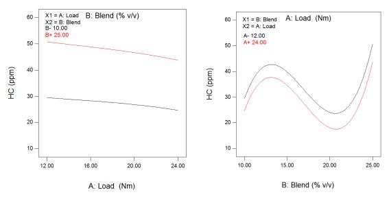
Fig. 4.33 Variation in HC with load and n-butanol-diesel blends at minimum and maximum values
