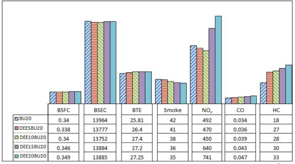
Fig. 4.114 Performance and emission of Diethylether-BU20 blends (100% rated power)<sup>3</sup>
