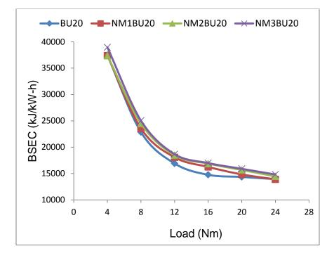
Fig. 4.60 (b) Variation of BSFC with engine load for NM-BU20 blends
