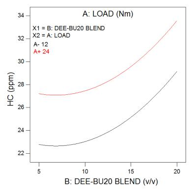
Fig. 4.113 Variation in HC with diethylether blending at medium and full load
