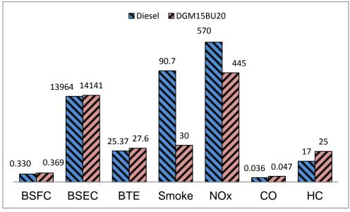
Fig. 4.125 Comparison of performance and emissions for diesel and DGM15BU20
