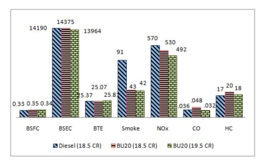
Fig. 4.51 Comparison of diesel and BU20 performance and emissions
