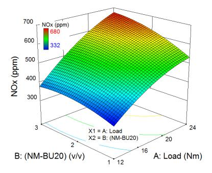
Fig. 4.67 Variation in NO<sub>x</sub> due to combined effect of load and NM blending
