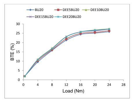
Fig. 4.104 Variation of BTE with engine load for Diethylether-BU20 blends
