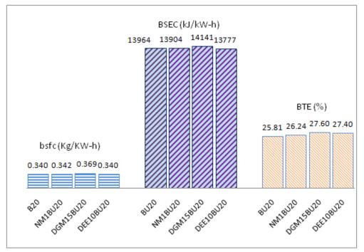
Fig. 4.122 Comparison of BSFC, BSEC and BTE at full load for different blended fuels<sup>4</sup>
