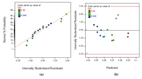
Fig. 4.9 (a) Plot of normal % probability vs. internal studentized residuals for CO (b) Plot of internal studentized residuals vs. predicted response for CO
