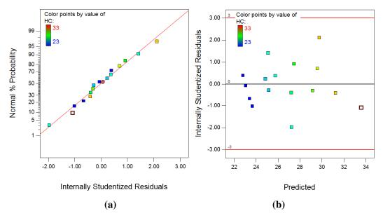
Fig. 4.99 (a) Plot of normal % probability vs. internal studentized residuals for HC(b) Plot of internal studentized residuals vs. predicted response for HC
