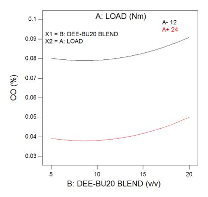
Fig. 4.111Variation in CO with diethylether blending at medium and full load
