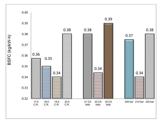
Fig. 4.41(a) BSFC at different CRs, injection timings and injection pressures for BU20
