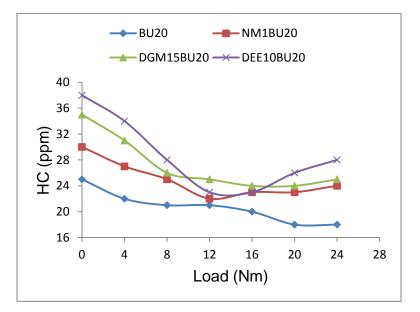
Fig. 4.121 Variation of HC with engine load for different blended fuels
