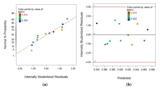
Fig. 4.52 (a) Plot of normal % probability vs. internal studentized residuals for BSFC(b) Plot of internal studentized residuals vs. predicted response for BSFC
