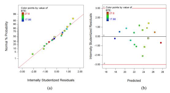
Fig. 4.74 (a) Plot of normal % probability vs. internal studentized residuals for BTE(b) Plot of studentized internal residuals vs. predicted response for BTE
