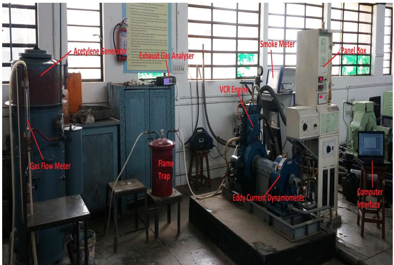
Fig. 3.12 Pictorial view of experimental setup
