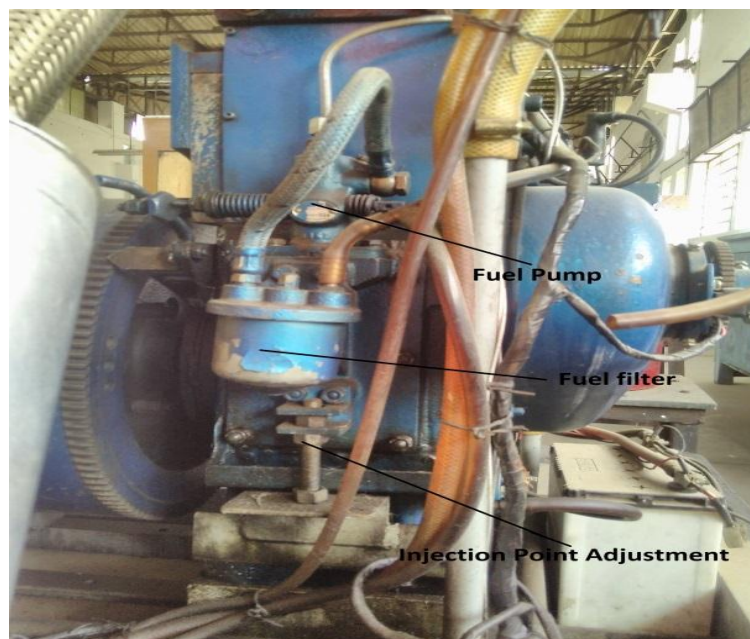
Fig. 3.9 Injection timing (IT) adjustment mechanism
