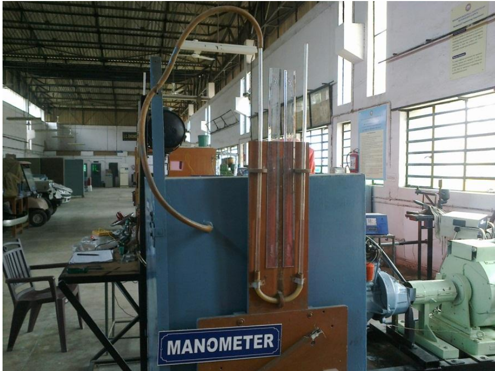
Fig. 3.4 U-tube manometer to measure the pressure drop in air box
