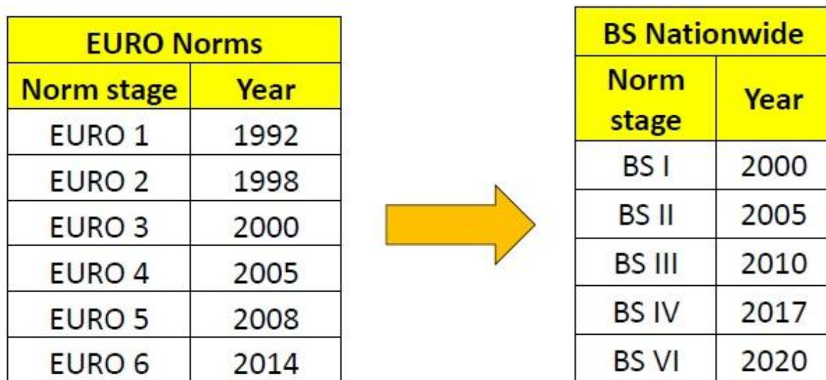
Fig. A.3 Comparison of implementation schedule of various Euro and BS norms [6]
