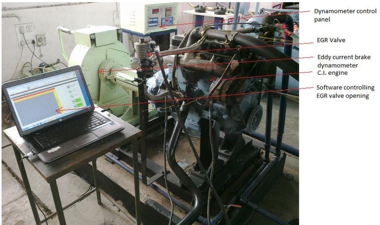
Fig. 3.15 Laboratory set-up showing the diesel engine, dynamometer, dynamometer panel, EGR valve and laptop (software) controlling EGR valve opening [32]
