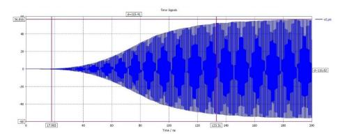
Fig. 5.14: Output port signal showing 1.61 kW RF power
