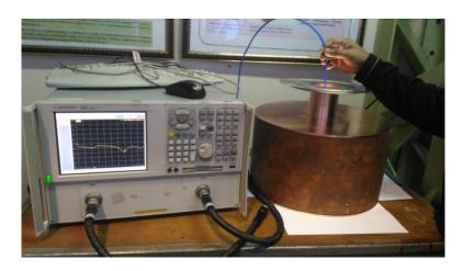
Fig. 7.21: Measurement of resonant frequency for the cavity assembly
