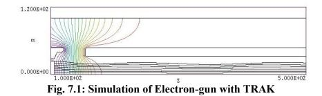
The Fig 7.1 shows the laminar flow of electron trajectories under the applied magnetic field of about 200 Gauss which is computed by using Brillouin formula [40]. The simulated value of beam current is 6.98 A in Trak. The design of electrodes optimized through TRAK has been re-simulated in MAGIC for cross-validation, as shown in Fig. 7.2.
