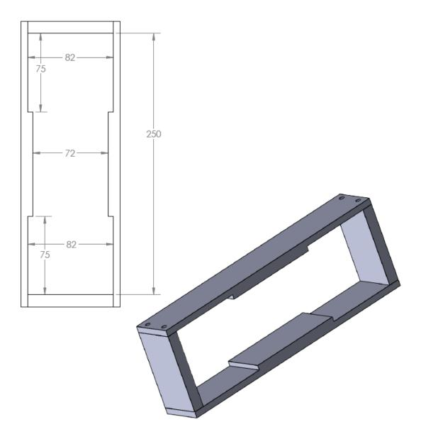
Fig. 6.20: Engineering design of the sheet beam cavity
