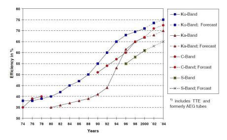
**Fig. 1.4: Progress in efficiency for Thales satellite TWTs over the years** (Source: From History to Future of Satellite TWT Amplifiers" Dr. Günter Kornfeld ;
