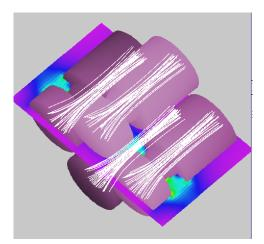
Fig. 1.12: A multi beam electron gun
