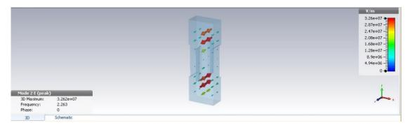
Fig. 6.27: Simulation of SBK cavity for its second mode frequency
