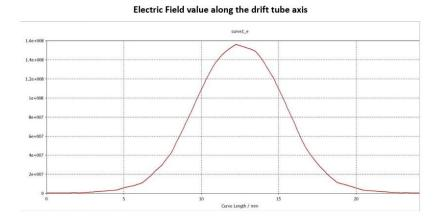
Fig. 4.3: The plot of Electric field along one drift tube axis
