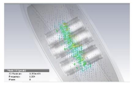
Fig. 4.2: Electric field across the cavity gaps
