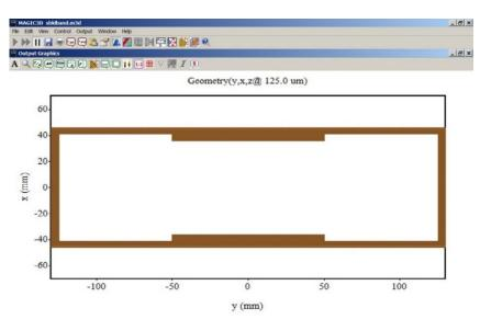
Fig. 6.17: Sheet beam cavity geometry in MAGIC-3D
