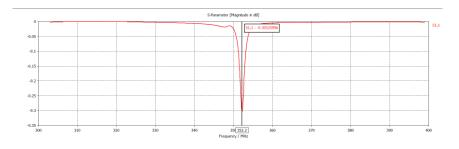
Fig 7.11: Plot of S<sub>11</sub> parameter vs Frequency for the input cavity
