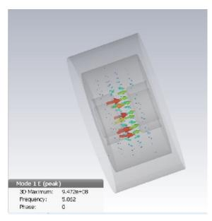
Fig. 2.4: Eigen mode simulation result for C-band cavity
