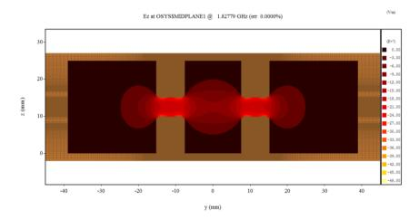
Fig. 4.5: Eigen mode simulation of RF cavity in MAGIC (the eigen mode frequency 1828 MHz)
