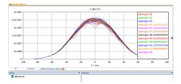
Fig. 6.8: The field profile with side height varying
