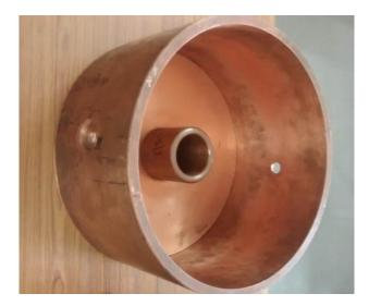
Fig. 7.18: The input cavity under development
