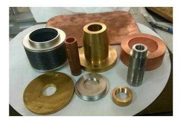
Fig. 7.19: The fabricated tuner parts
