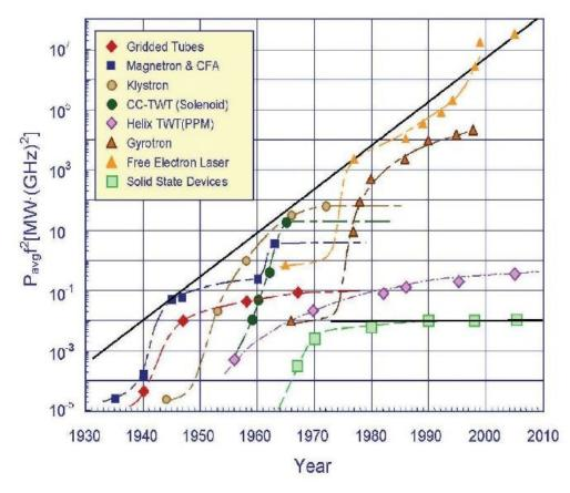
**Fig. 1.3: Progress in factor 'Pf<sup>2</sup> for vacuum electronics over the years** *(Source: Vacuum Electronics: Status and Trends, Baruch Levush etal.)*
