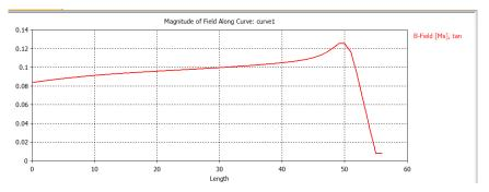
Fig. 3.12: The simulated magnetic field vale at drift tunnel axis
