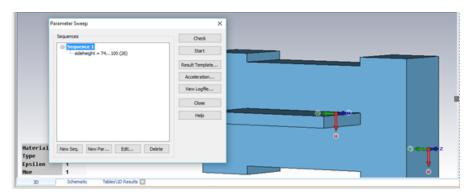
Fig. 6.7: Parameter optimization for quarter wave section height
