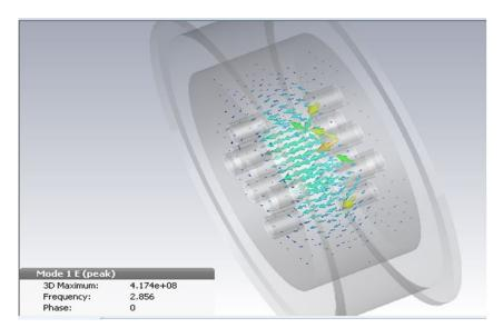
Fig. 2.8: The Eigen Mode frequency 2.856 GHz found in CST
