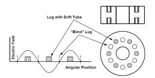
Fig. 2.2: Cross section of HM MBK (Source: A.S Gilmour, Klystons, TWTs, Crossed-Field Amplifier and Gyrotrons)
