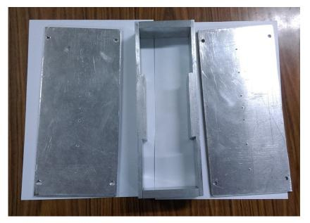
Fig. 6.21: Fabricated sheet beam cavity
