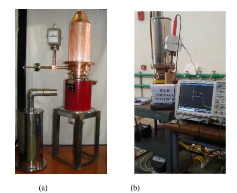
Figure 7.27. (a) Developed beam stick tube along with electromagnet (b) Hot testing of beam stick tube
