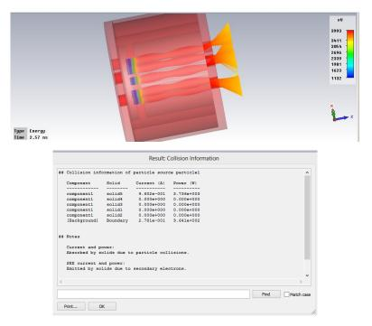
Fig. 3.18: Electron trajectories and collision information after simulation
