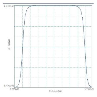
Fig. 3.3: The simulated magnetic field in Trak
