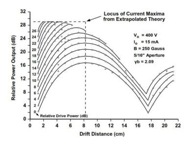
Fig. 5.1: Optimum distance between buncher cavity and output cavity from Mihran's experiment (Source: T.G. Mihran,, IRE transactions on electron devices, January 1959)
