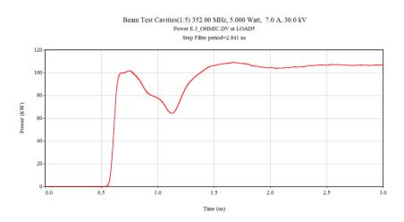
Fig. 7.13: Simulation of RF output power
