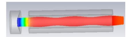
Fig. 3.4: The simulated electron trajectories in CST
