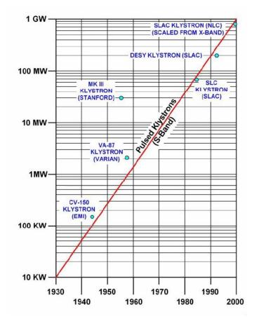
**Fig. 1.11: Klystron power growth over the years since its invention** (*Source: High Power Klystrons: Theory and Practice at the Stanford Linear Accelerator Center, G Caryotakis*)
