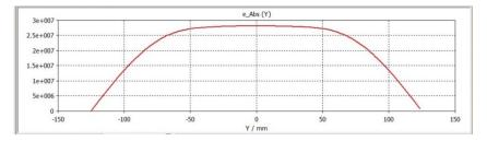
Fig. 6.13: The flat field profile after optimization
