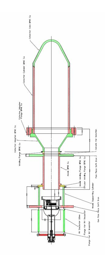
Fig. 7.26: Schematic of the beam stick tube
