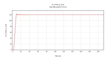
Fig. 7.9: Simulation result for R/Q of the input cavity
