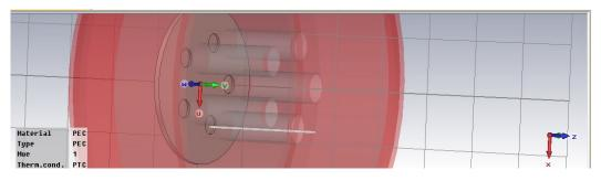
Fig. 7.32: Geometry of the five beam electron gun
