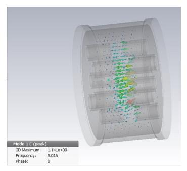
Fig. 2.7: The Eigen Mode frequency 5 GHz found in CST
