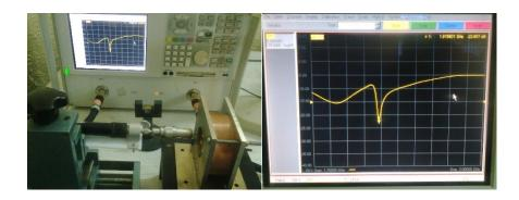
**Fig. 4.7: Characterization of the five beam cavity** (the measured resonant frequency is 1815 MHz)
