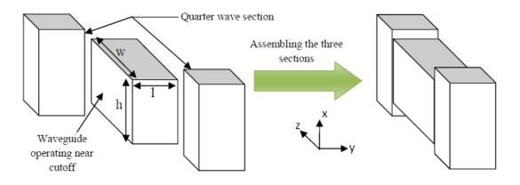
Fig. 6.3: Barbell cavity showing the middle waveguide section and the two quarter wave section
