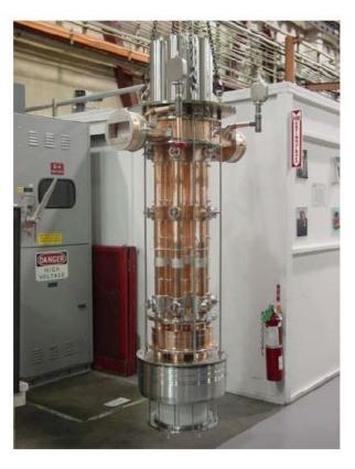
Fig. 1.17: The Thales MBKFig. 1.18: The CPI MBK(Source: High Power Klystrons: Theory and Practice at the Stanford Linear Accelerator<br/>Center, G Caryotakis)
