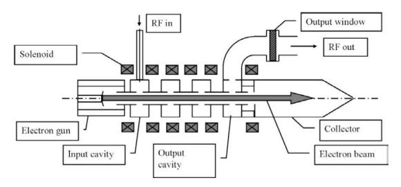
**Fig. 1.6: Schematic Diagram of Single Beam Multi cavity Klystron** (Source: Google images; Radio Frequency Power Generation, R. G. Carter)
