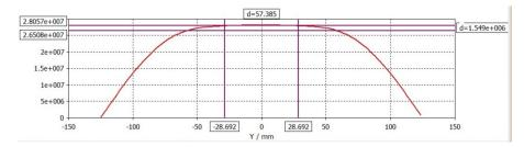
Fig. 6.15: The flat field profile along beam width of 50.4 mm
