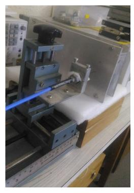
Fig. 6.25: SBK cavity excited through end
