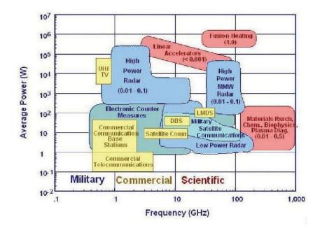
Fig. 1.2: Applications of high power microwave sources
