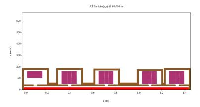
Fig. 7.12: Beam wave interaction simulation in MAGIC 2D
