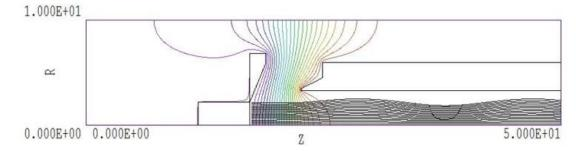
Fig. 3.2: The simulated electron gun in Trak
