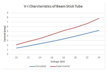
Fig.7.28 Measured Characteristics of beam stick tube
