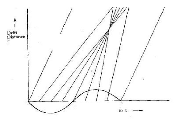
**Fig. 1.8: Applegate diagram for electrons in a field free drift region** (Source: Power Klystron Today, Smith, Phillips)
