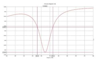
Fig. 7.16: S-parameter plot of output cavity
