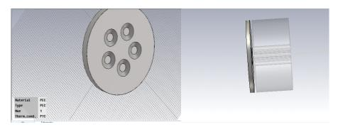
Fig. 3.6: Geometry of the five beam electron gun
