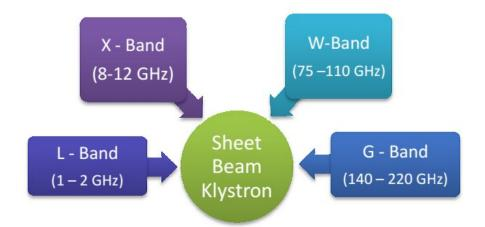
Fig. 1.19: Frequency bands over which the SBK research is being carried out
