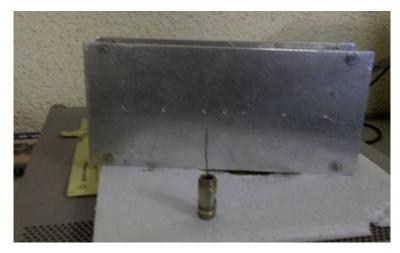
Fig. 6.22: Probe antenna with assembled sheet beam cavity
