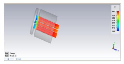
Fig. 3.7: Beam Trajectories with focusing magnetic field
