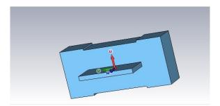
Fig. 6.4: Modelling of a SBK cavity in CST Microwave Studio
