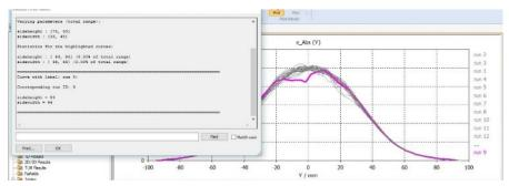
Fig. 6.12: The field profile with side height = 84 mm, side width = 44mm
