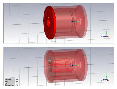
Fig. 3.11: Electron gun modelled with electromagnet
