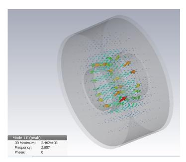
Fig. 2.5: Simulation of frequency for the S-Band Klystron
