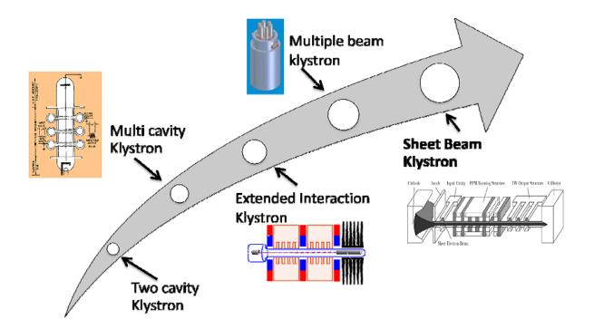
Fig. 1.16: Various phases in the Klystron technology
