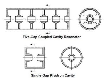
Fig. 1.15: Five-gap Vs Single-gap Klystron Cavity
