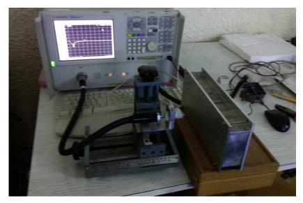
Fig. 6.23: Cold test set-up for measuring the frequency of SBK cavity
