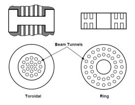
**Fig.2.1: Cross section of FM MBK** (Source: A.S Gilmour, Klystons, TWTs, Crossed-Field Amplifier and Gyrotrons)
