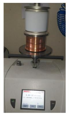
Fig. 7.3: Leak testing of Electron Gun
