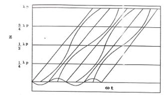
**Fig. 1.9: Modified Applegate diagram showing the effect of space charge** (Source: Power Klystron Today, Smith, Phillips)
