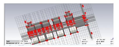
Fig. 5.9: RF interaction region along with mesh view
