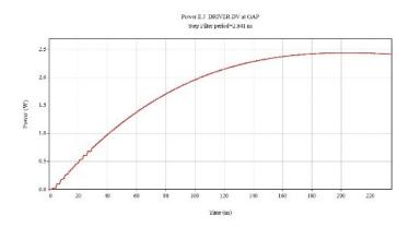
Fig. 7.14: Simulated RF input power
