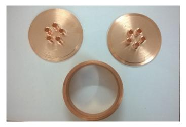
Fig. 4.6: The piece parts of a five beam cavity
