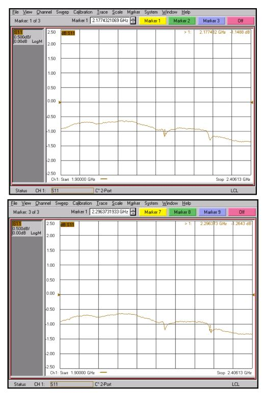
Fig. 6.26: Measured resonant frequencies for first two modes of the cavity
