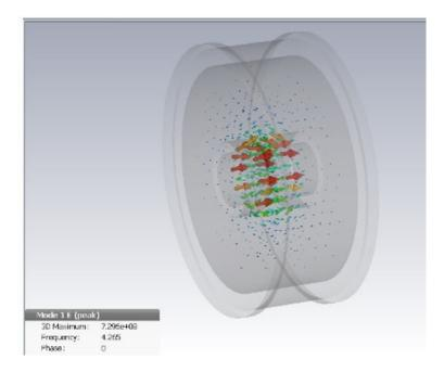
Fig. 2.3: Simulation result of cavity in CST Microwave Studio
