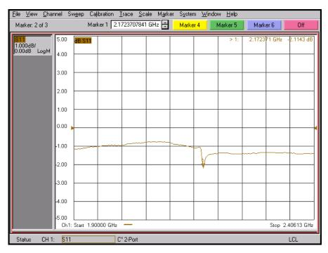
Fig. 6.24: Measured resonant frequency of SBK cavity
