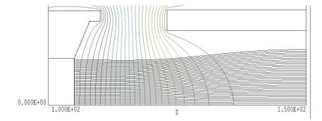
Fig. 7.30: The simulated electron gun in TRAK
