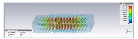
Fig. 6.14: The eigen mode frequency after optimization
