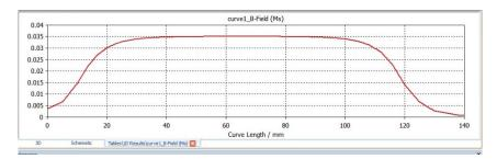
Fig.7.33: Simulated value of Magnetic Field on Drift tube axis
