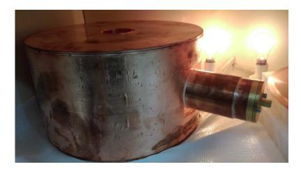
Fig. 7.20: Final cavity assembly with tuning mechanism
