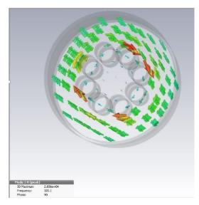
Fig 3.21: The Magnetic Field lines after eigen mode simulation
