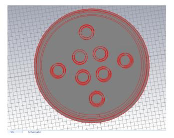
Fig. 2.6: Placement of the drift tubes
