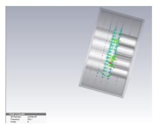
Fig 3.20: The Eigen Mode frequency 325 MHz found in CST
