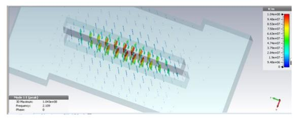
Fig. 6.5: Eigen mode simulation in CST Microwave Studio
