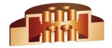
Fig. 1.13: A multi beam klystron cavity
