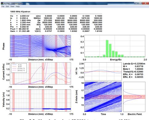
Fig. 5.3: Simulation in AJDISK (output power 68 W)
