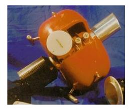
Fig. 3.1: One kW (CW) power klystron
