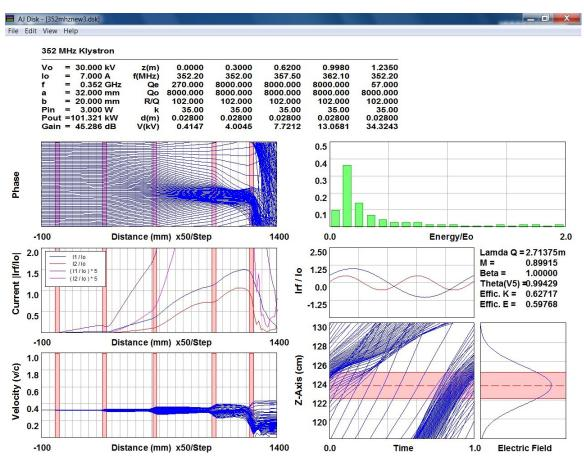
Fig. 7.4: Simulation of output power in AJDISK code (simulated power 101 kW)
