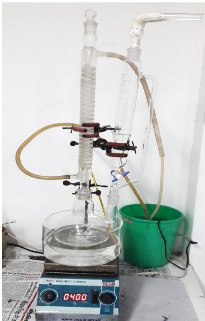
Figure 4.2 Photograph of the experimental setup for the synthesis of ionic liquids
