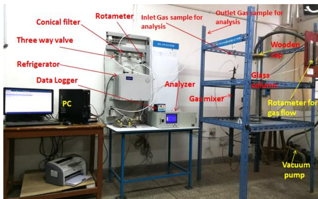
Figure 4.7 Photograph of the experimental setup used for desulfurization of the gaseous mixture
