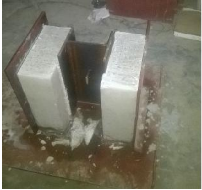
Fig. 3.24 Demoulding of specimen
