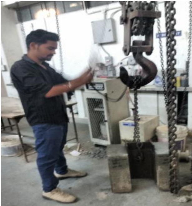
Fig. 3.25 lifting of specimen by gantry girder
