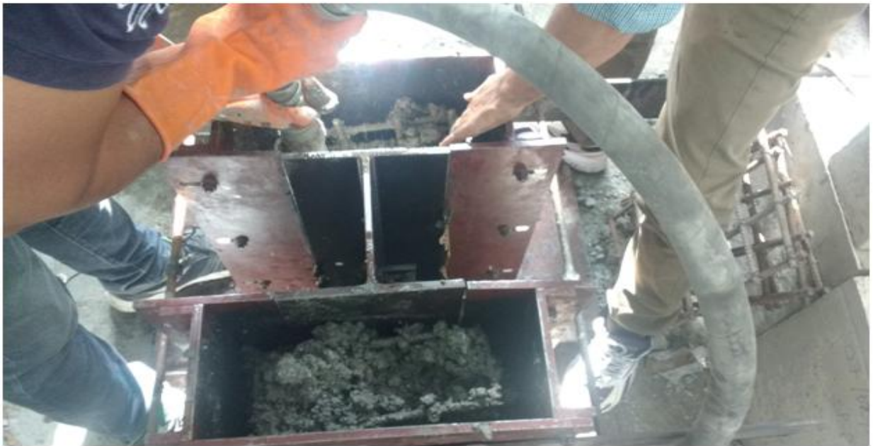
Fig. 3.22 Compaction carried out with the help of needle vibrator
