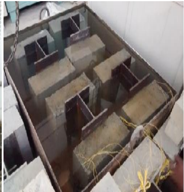
Fig. 3.26 Curing of specimens in tank
