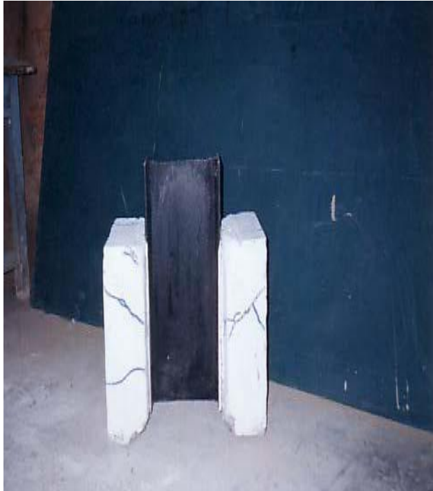
Fig2.2: Cracks of the concrete slab near the position of the studs shear connector (Abbas et al. (2005))
