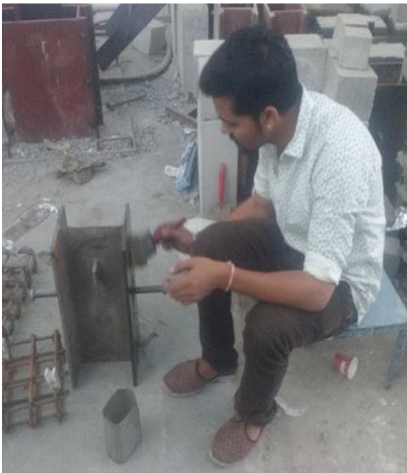
Fig.3.18 Oiling of Flange section to avoid Frictional resistance
