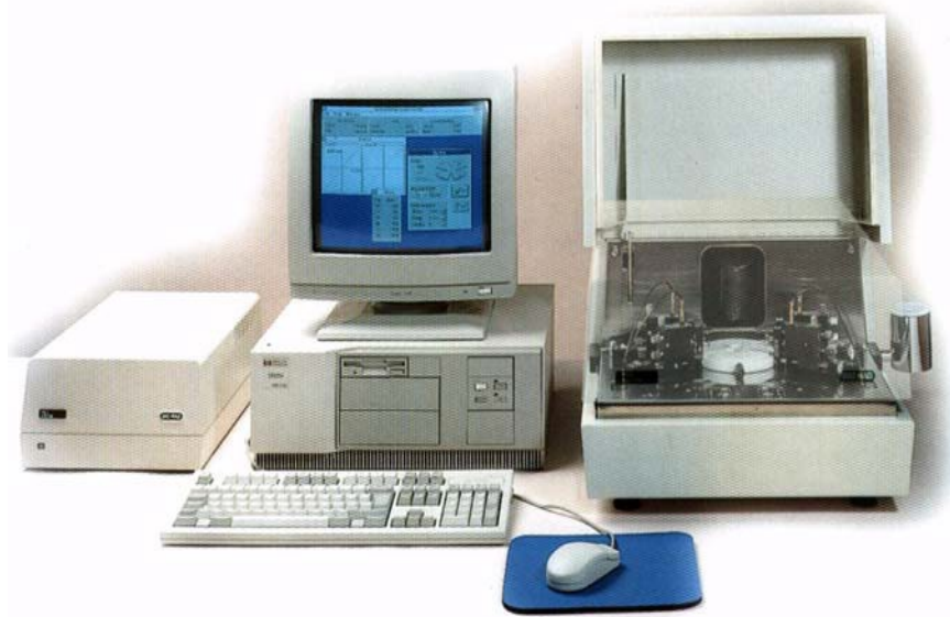
Figure 6.4 Hall Effect Measurement System HL 5500 PC (Nanometrics)
