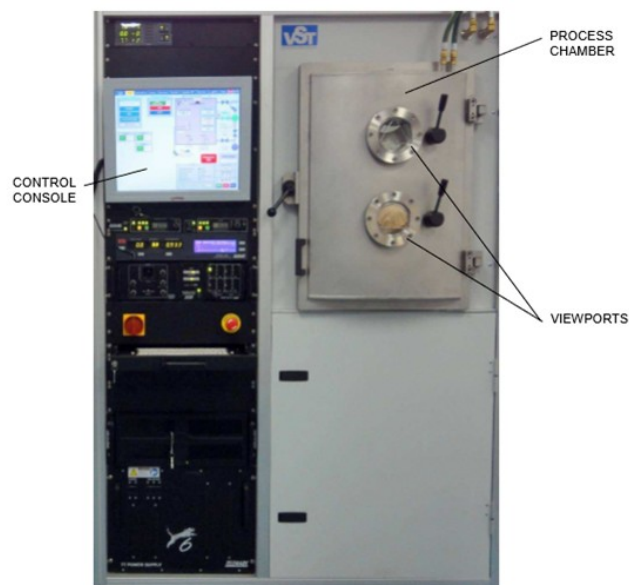
Figure 5.8 The TFDS-462B thin film deposition system
