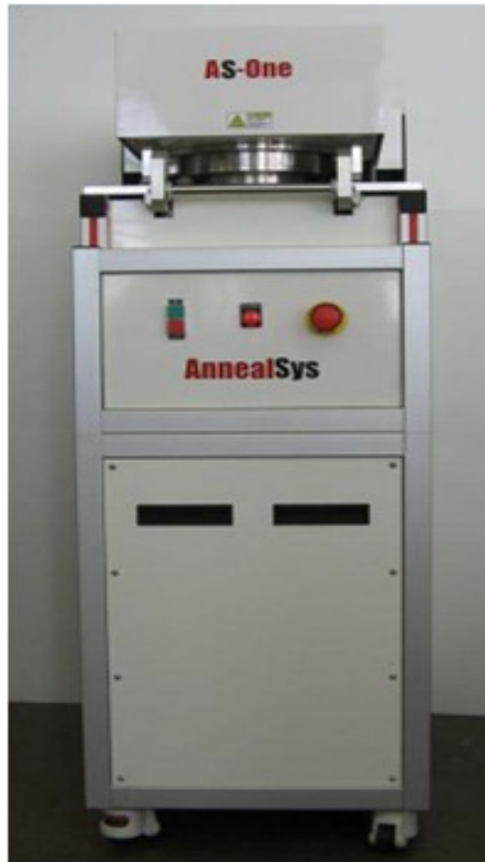
Figure 5.3 Rapid Thermal Annealing system at ODG, CEERI, Pilani
