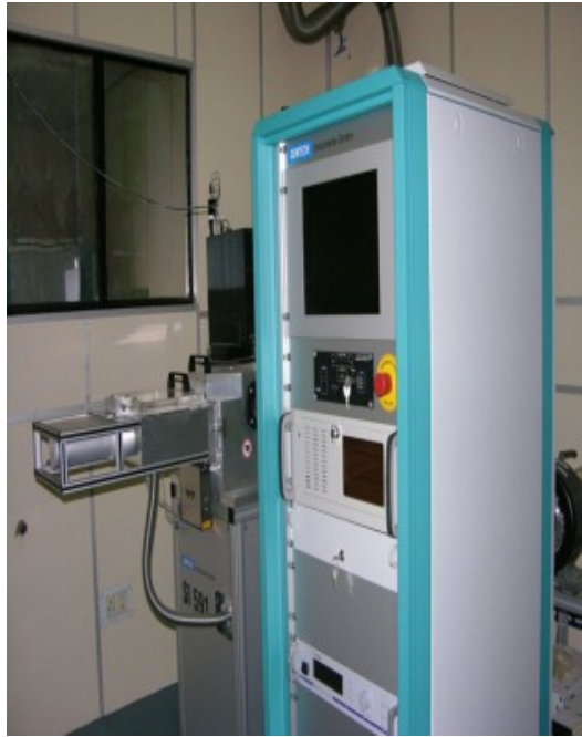
Figure 5.6 Reactive Ion Etching (RIE) system at ODG-CEERI, Pilani
