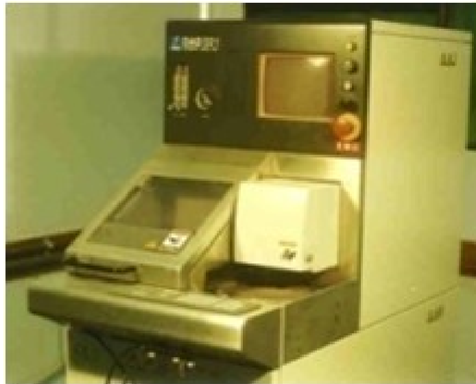
Figure 5.2 Automatic Dicing Saw (DAD-321) system
