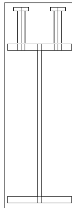
Figure 3.9 Partitioned I-section along with shear studs
