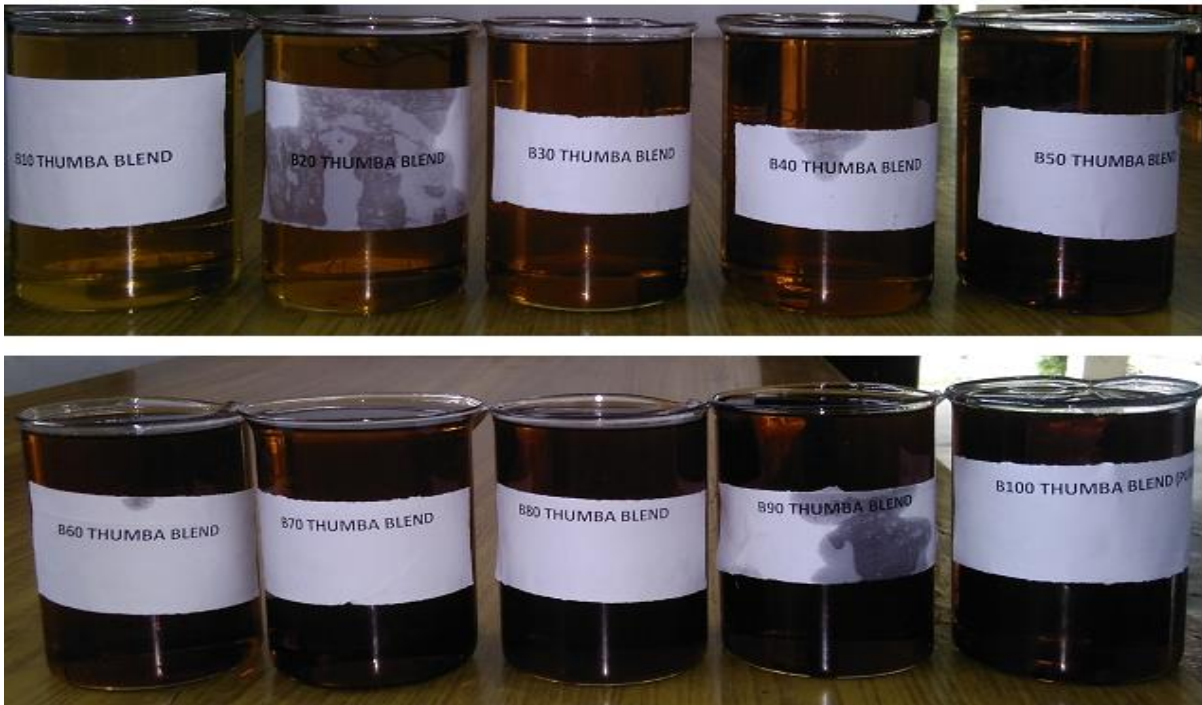
Figure 3.6 Developed Thumba oil blends with diesel
