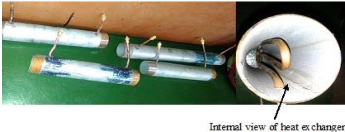
Figure 3.4 Developed heat exchangers
