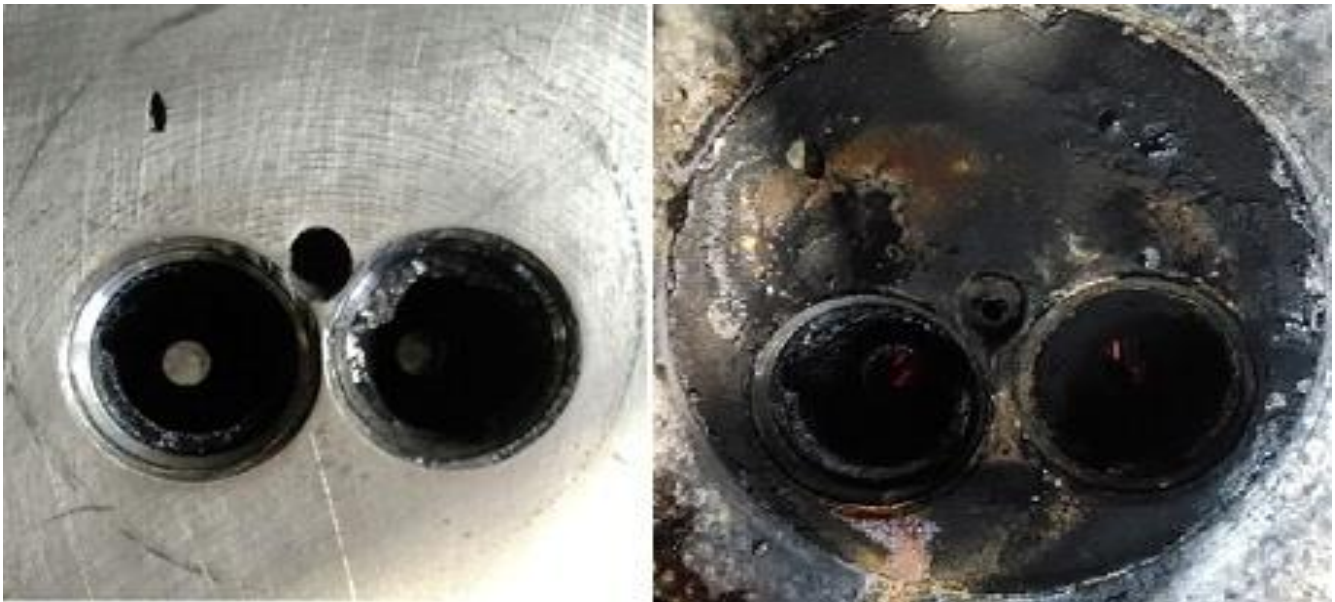
Engine Head before the test
