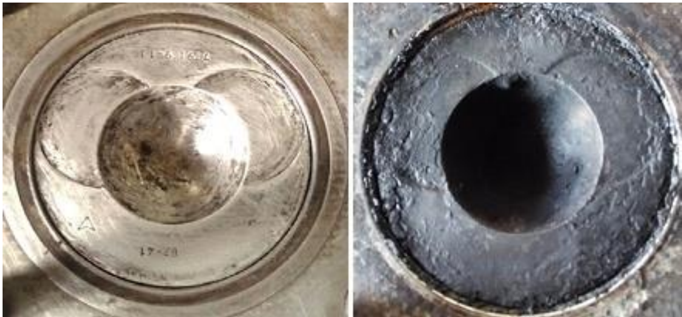
Top of piston before the test
