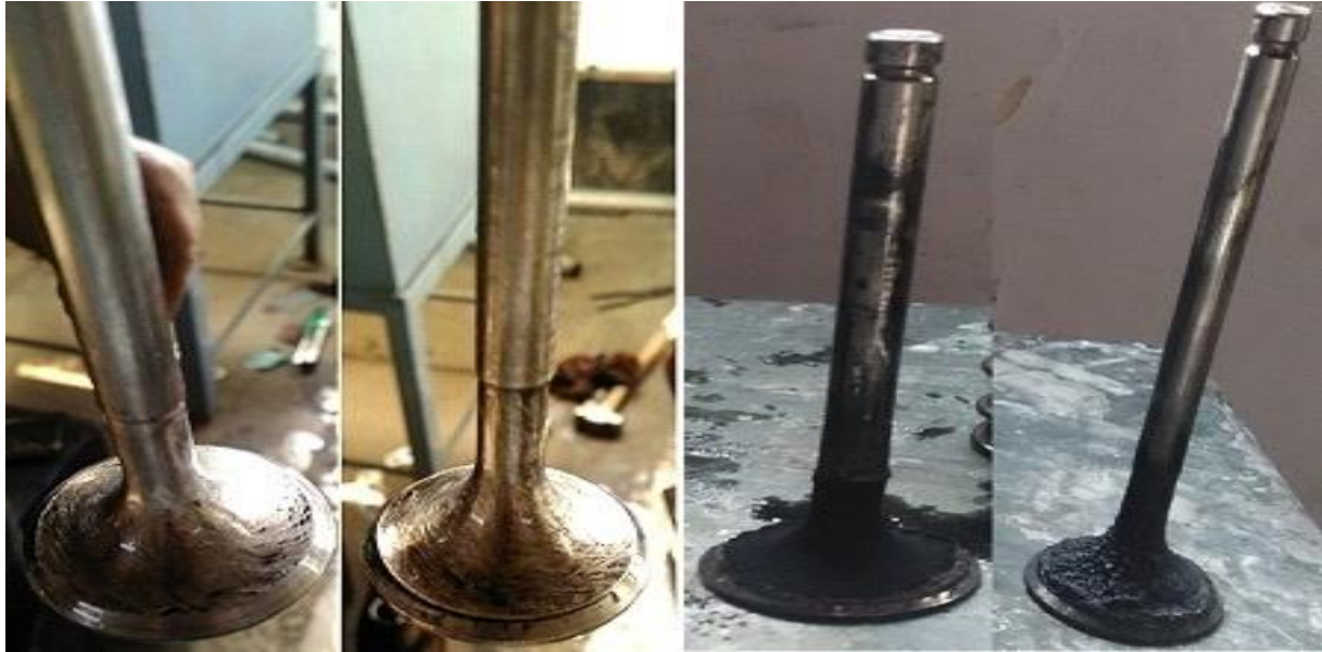
Engine Suction and Exhaust Valve before the test
