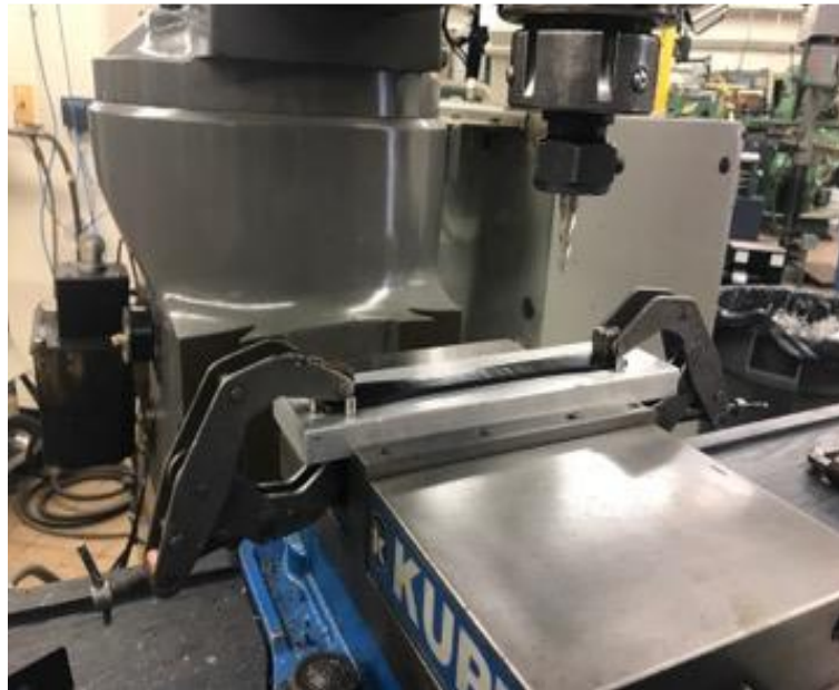
Figure 4.11 Milling the Edges of a Molded Tensile Bar
