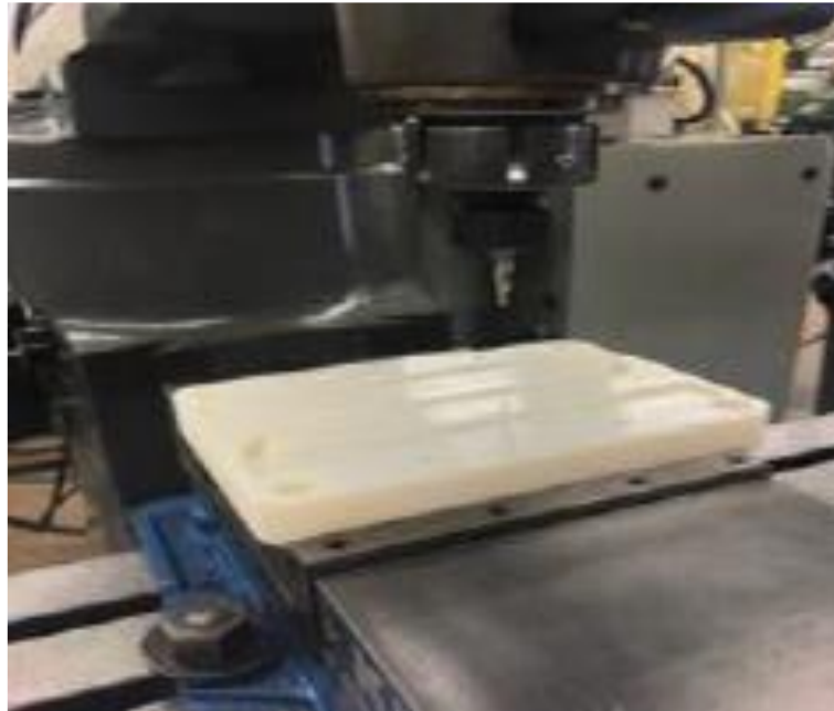
Figure 4.10 CNC Bridgeport Mill used to post process the Digital ABS mold and tensile
