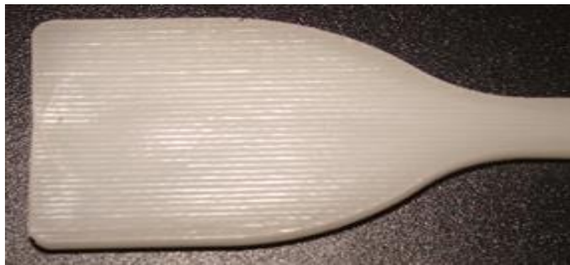
Figure 4.15 Surface details of the tensile sample after 6 shots
