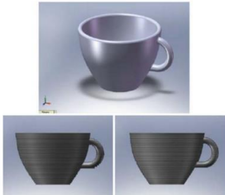
Figure 1.5 Layer by Layer depositions to build a product (Prest et.al, 2013)
