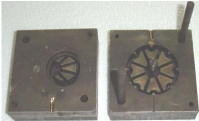
Figure 2.2 Metal mold used in injection molding (Dickens, 1997)
