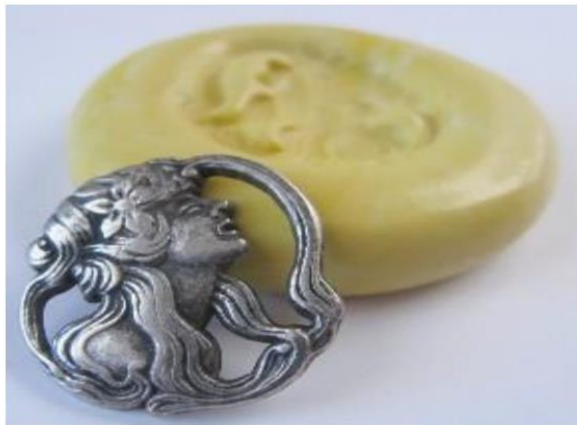
Figure 1.4 Example of silicon rubber soft tooling
