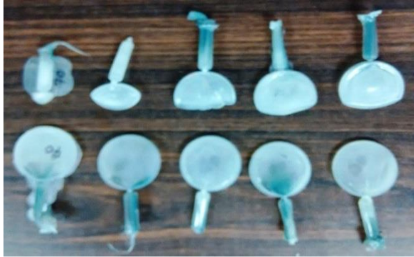
Figure 3.17 Progressive stages of the component made in the trial runs
