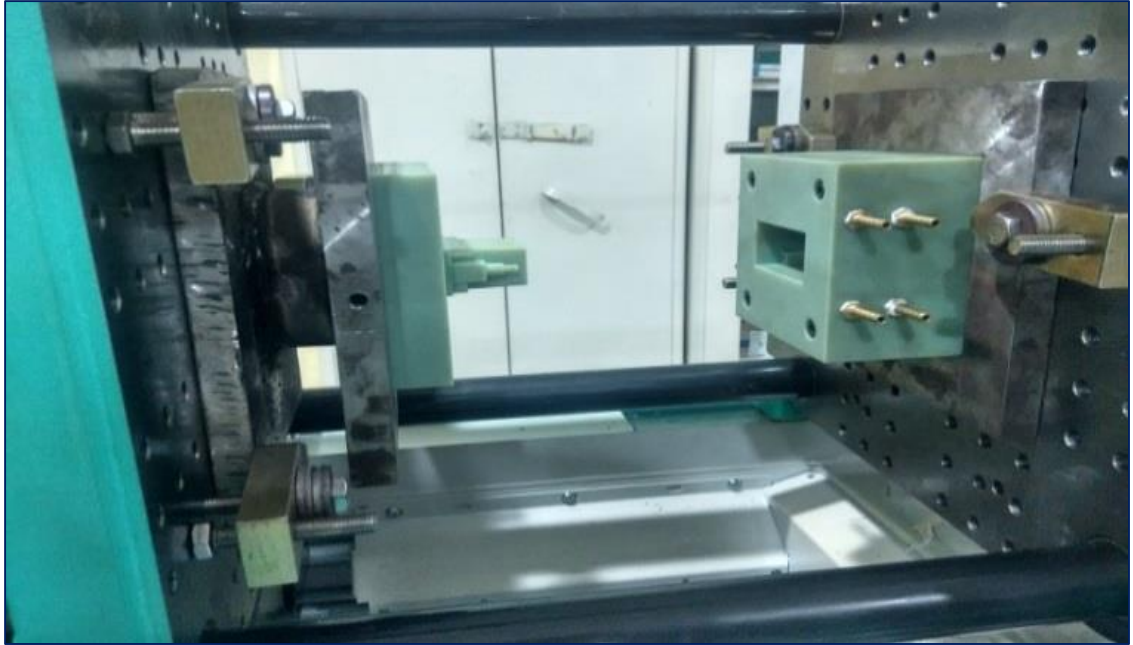
Figure 6.10 3D polyjet mold mounted on for experiment
