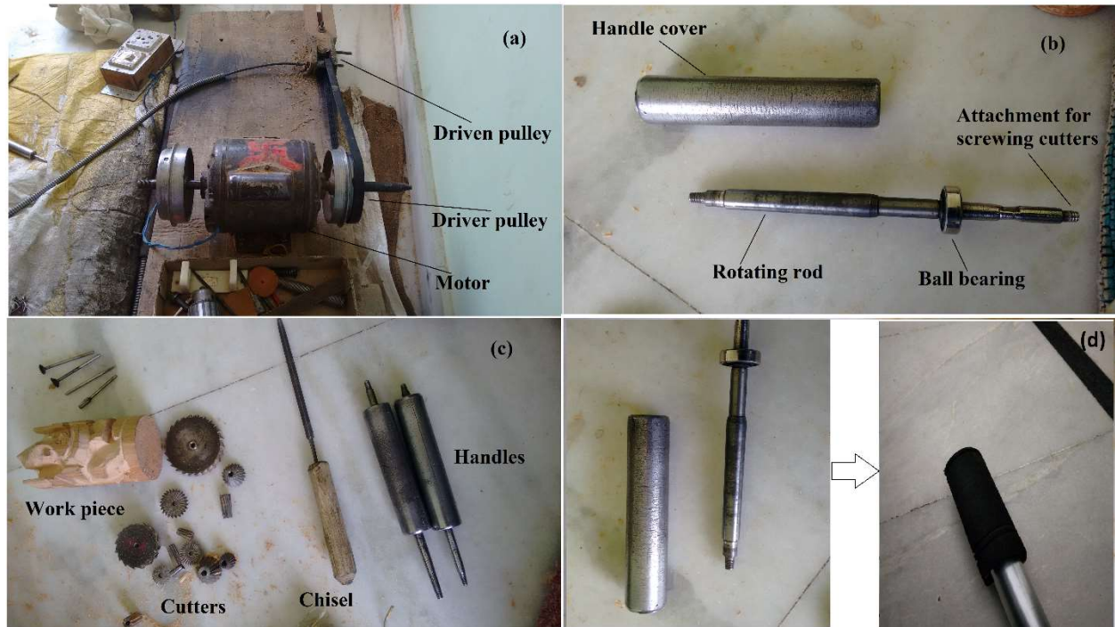
Figure 5.3.5. Physical structure of conventional wood carving tool arrangement. (a) Driving motor and pulley arrangement; (b) Carving tool handle; (c) Various cutters used during carving, chisel, tool handles and a wooden work piece; (d) Overall process of intervention for carving tool handle.
