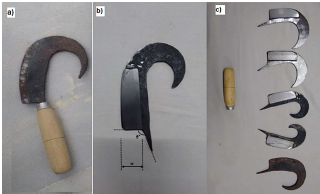
Figure 5.1.1. a) Conventional weaving knife; (b) Evaluation criteria for prototype intervention of knife blade and (c) pairs of knife blades used in the study.
