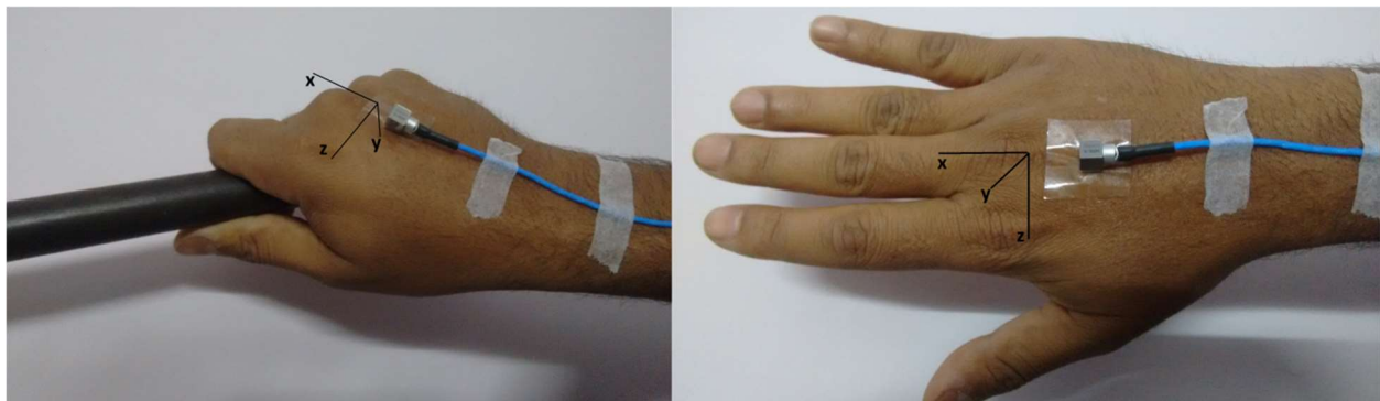
Figure 3.6. Orientation of accelerometer on workers hand.
