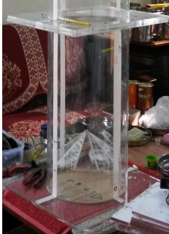
Figure 3.12: Construction of the column of the pilot plant at MNIT Jaipur campus
