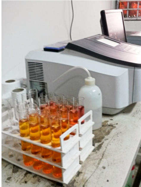
Figure 4.8: Testing for residual aluminium on Shimadzu UV 1800 spectrophotometer installed at the PHE lab
