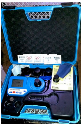
Figure 4.7: Portable HANNA ® spectrophotometer kit for testing chlorine in use on field
