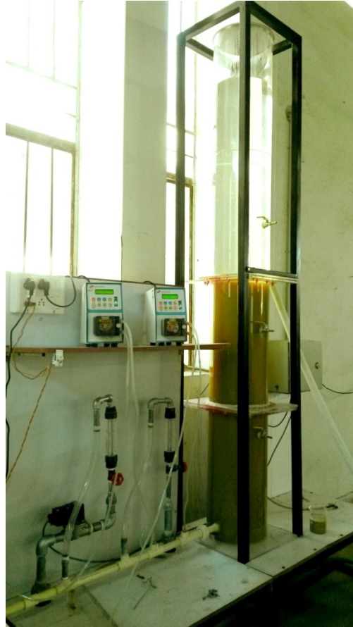
Figure 3.21: Development of the sludge blanket in the Superpulsator ® pilot plant
