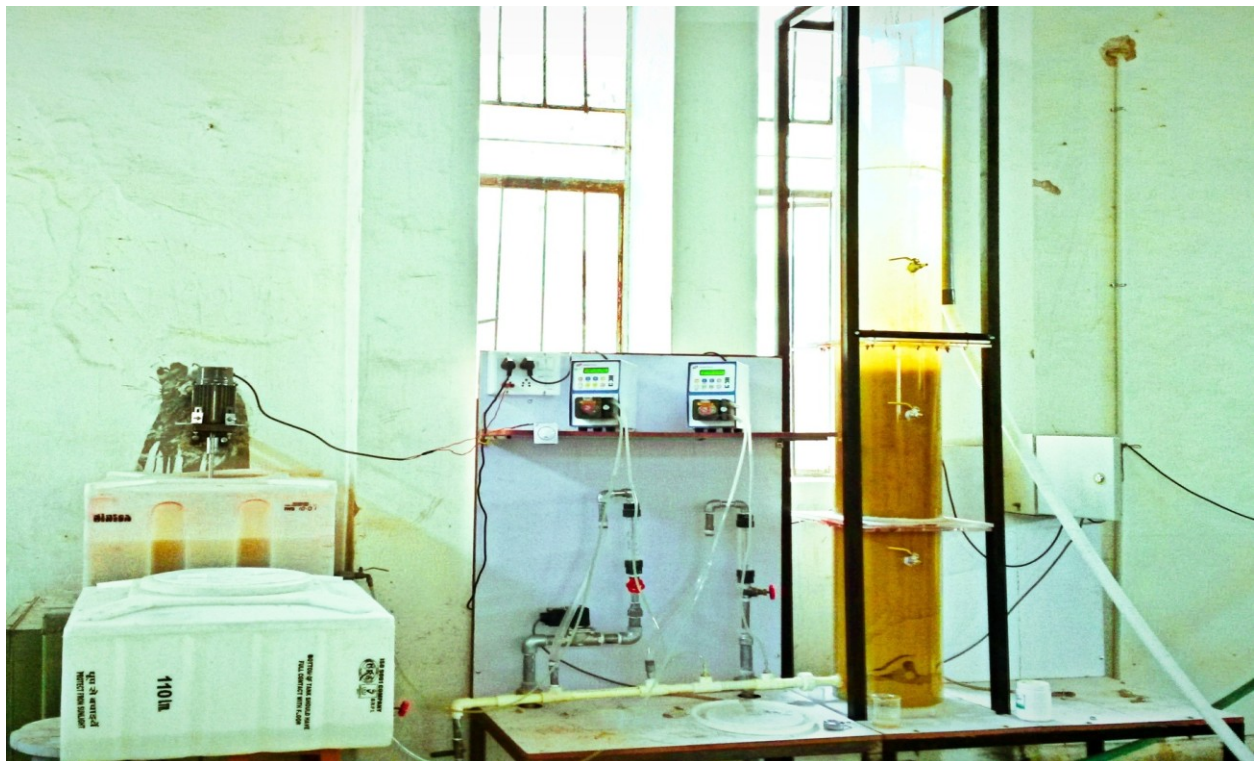
Figure 3.20: Pilot plant based on Superpulsator® technology is designed for a capacity of about 8000 liters per day and is installed in the Hydraulics lab of Malaviya National Institute of Technology, Jaipur.
