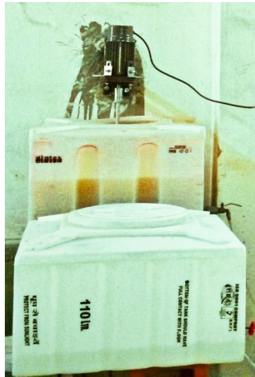
Figure 3.17: Two storage tanks of 100l capacity each, one of which is provided with a mechanical stirrer
