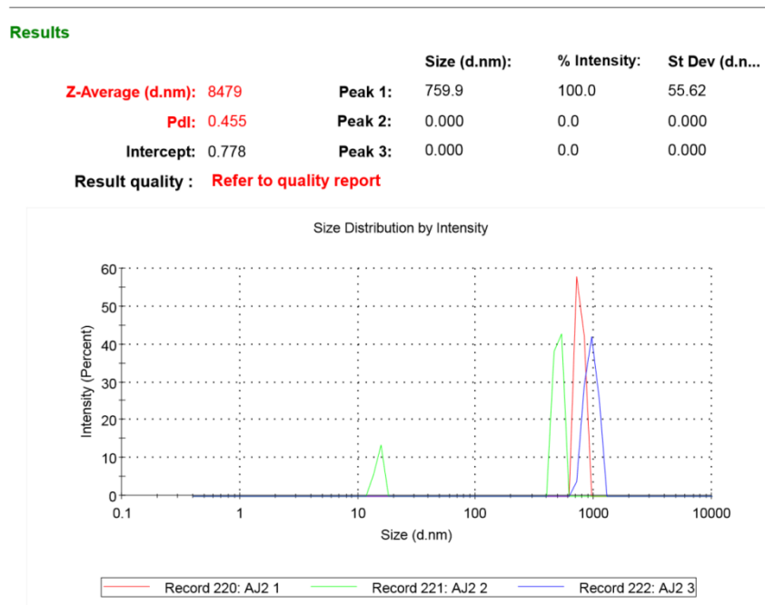
Figure 5.14: Particle size analysis of pre-chlorinated and coagulated Bisalpur water (unsonicated) with about 4 minute detention time after hydraulic jump as simulated
