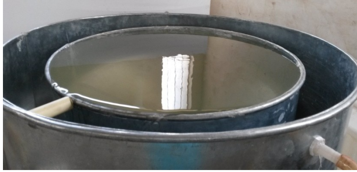
Figure 3.24: View of the top of the conventional clariflocculator
