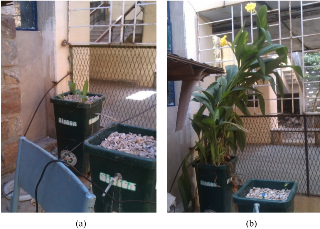
Fig. 3.5. Unit with different media configuration and gradation planted with Canna indica (UN-cn-sd) (a) at initial development stage and (b) at maturation stage
