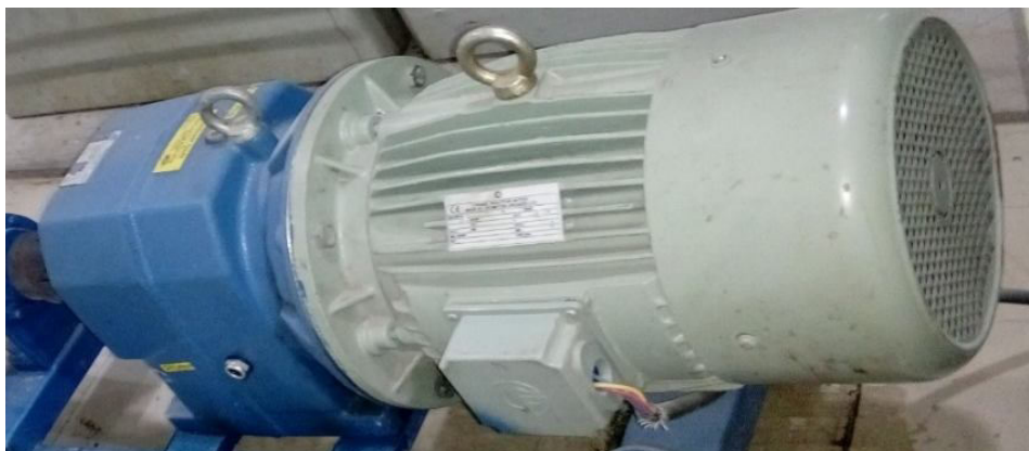
Figure 4.16 Electric motor with gear unit.
