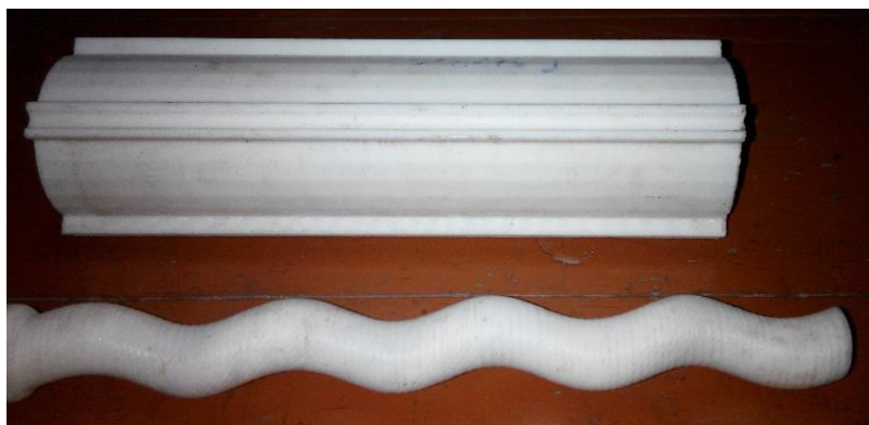
Figure 4.4 Fabricated rotor and stator parts of MUAFM
