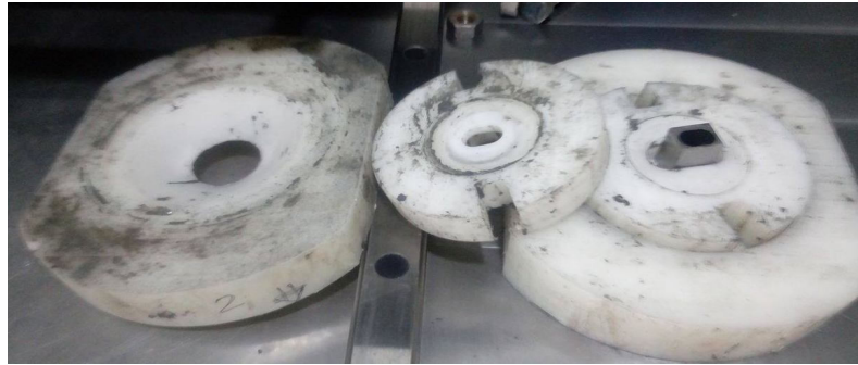
Figure 4.27 Nylon tooling for holding the stamping die in commercial AFM
