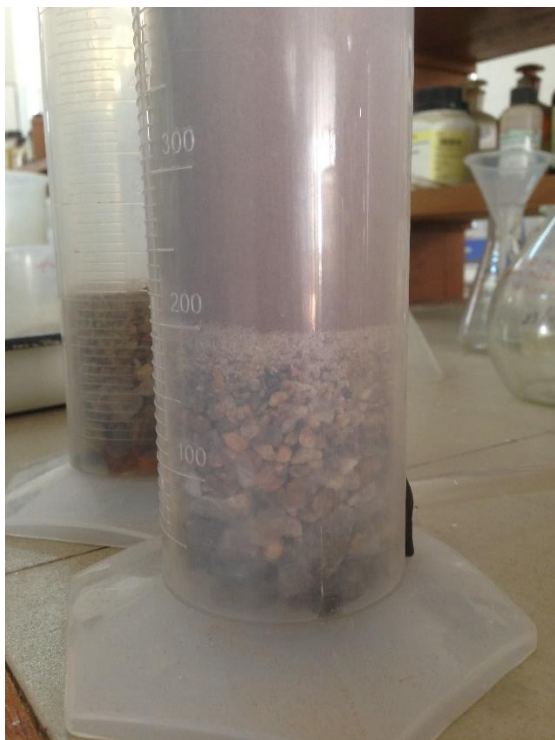
Figure 3.4. The sand and gravel layers in the filter bed
