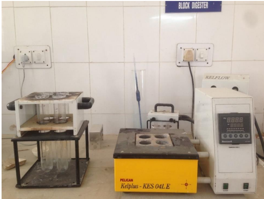
Figure 3.5. TKN Digestion assembly
