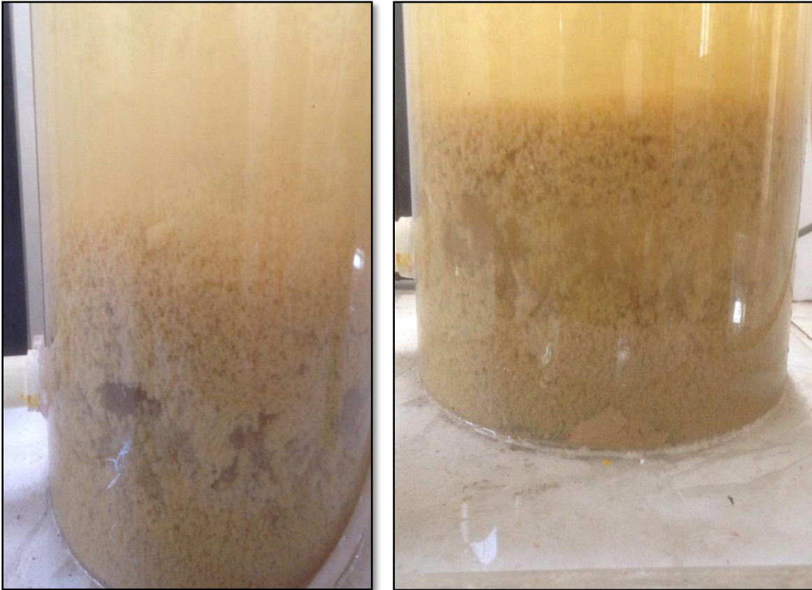
Figure 3.6: Photograph of blanket formation in Pulsator pilot plant
