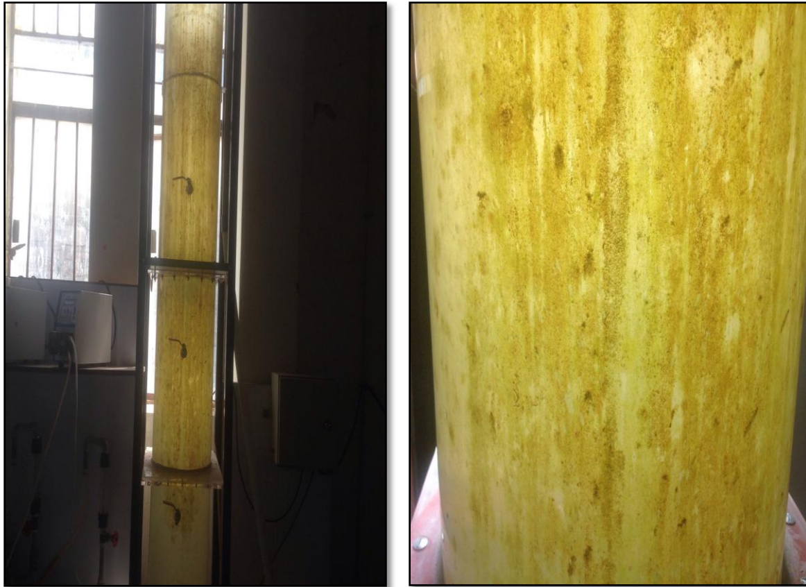
Figure 3.7: Algal growth in the pulsator pilot plant
