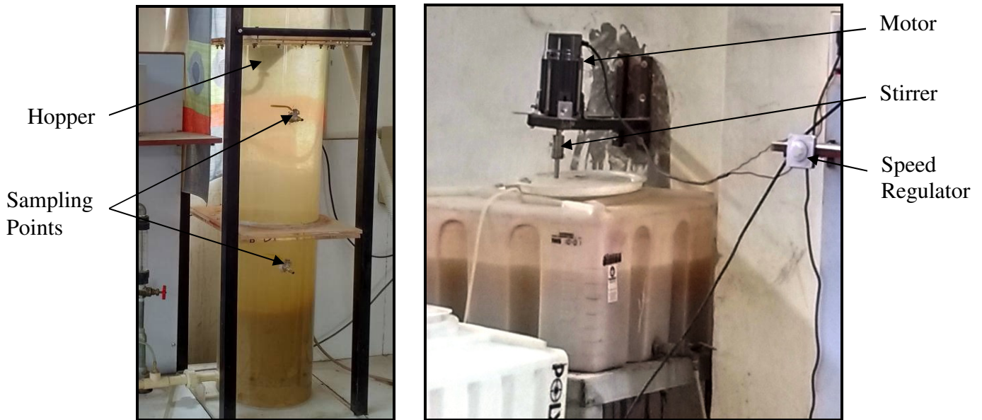
Figure 3.13: Pictures showing Sludge Extraction (Hopper) and Stirrer arrangements
