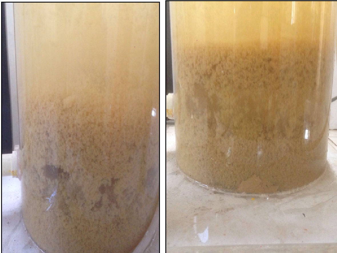
Figure 4.19: Photograph of blanket formation in Pulsator pilot plant
