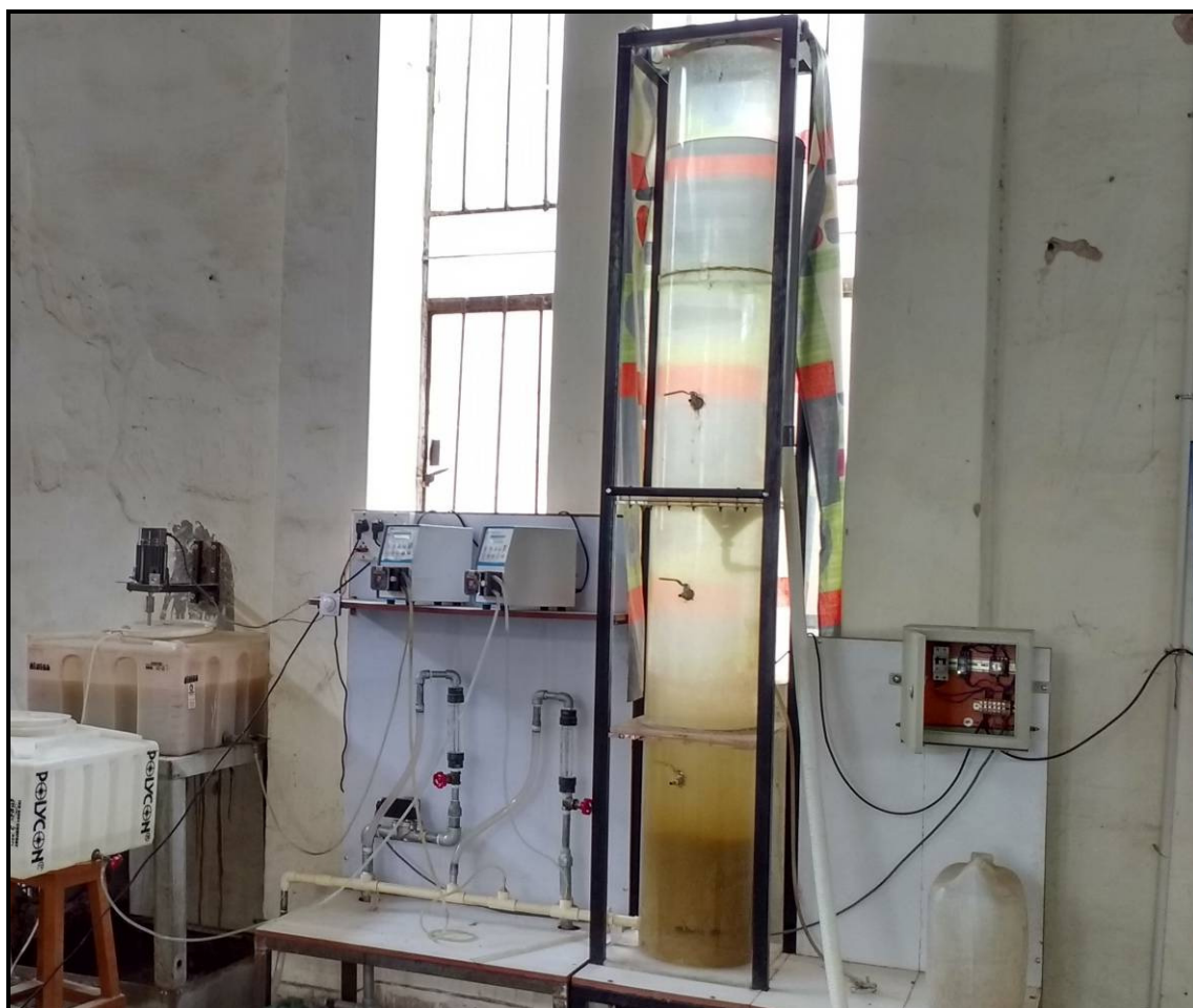
Figure 3.15: Photograph of the complete setup of the pulsator clarifier pilot plant
