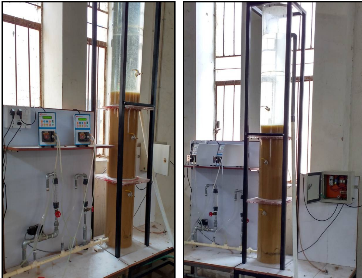
Figure 4.20: Pictures of Stable Sludge Blanket in its Full Experimental Height
