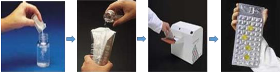
Figure 3.2: Stepwise procedure for estimating TCs detection using Colilert-18 Hr. Method with Quanti-Trays
