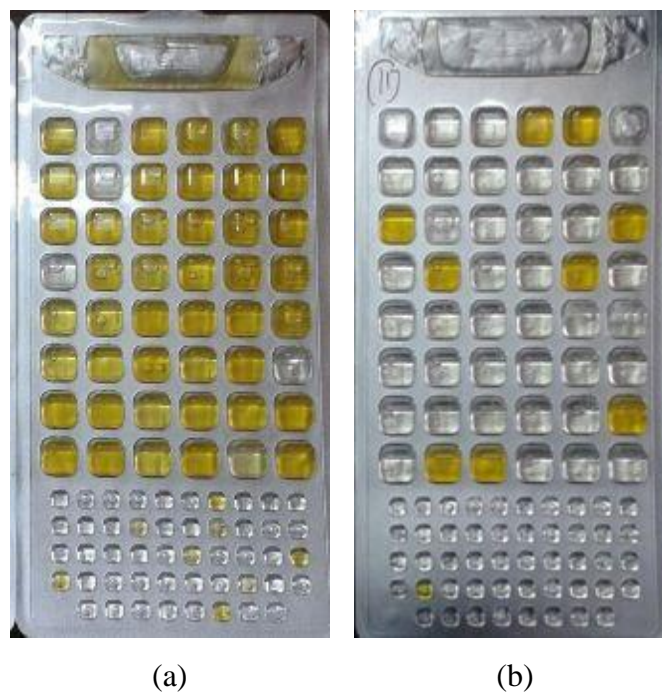
Figure B.2: Colilert results of ozonation showing removal of microbes in terms of MPN/100 mL (a) secondary treated effluent and (b) effect of 30 mg/L of TOD
