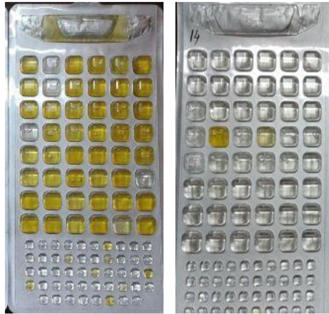
Figure C.2: Colilert results of UV disinfection showing removal of microbes in terms of MPN/100 mL (a) secondary treated effluent and (b) effect of UV dose 75 \text{ mJ/cm}^2
