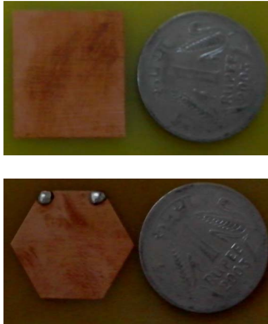
Fig. 5.16. (a) Side view of stacked antenna structure with shorting pin. (b) Top view of designed rectangular patch. (c) Top view of designed hexagonal patch with feed and shorting pin.
