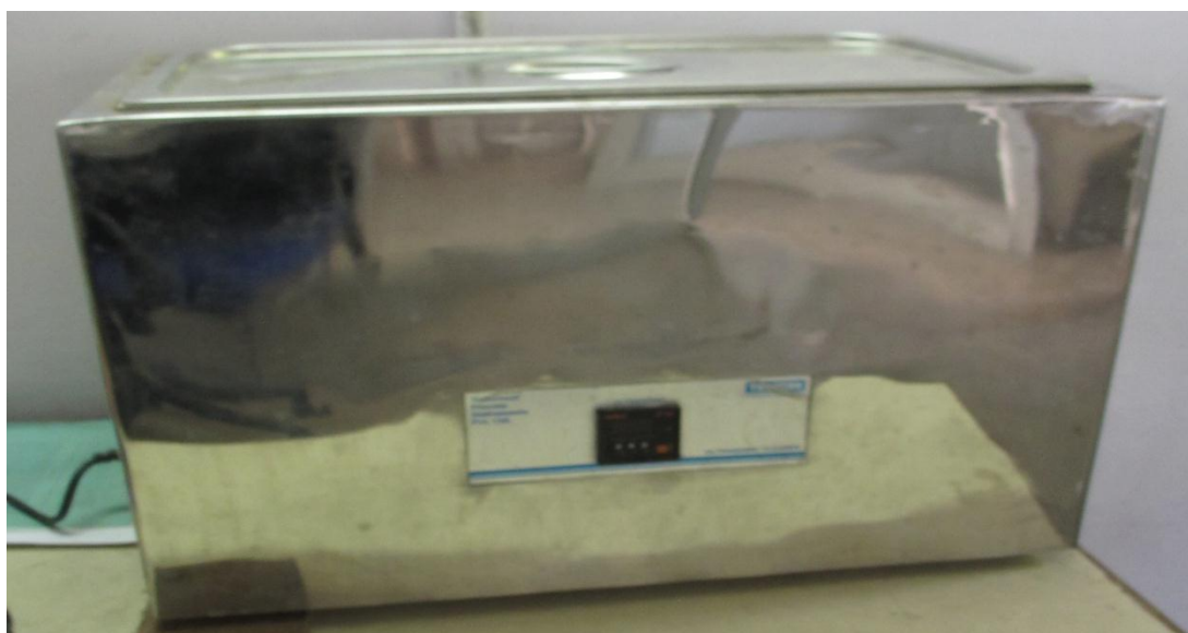
Fig. 3.7 Ultrasonic Cleaner apparatus for sonication
