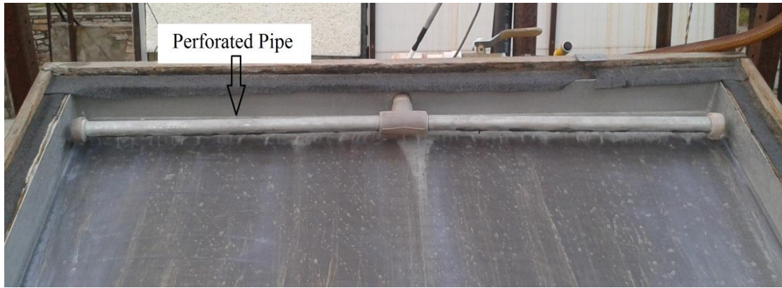
Fig. 4.8 Film formations using perforated pipe
