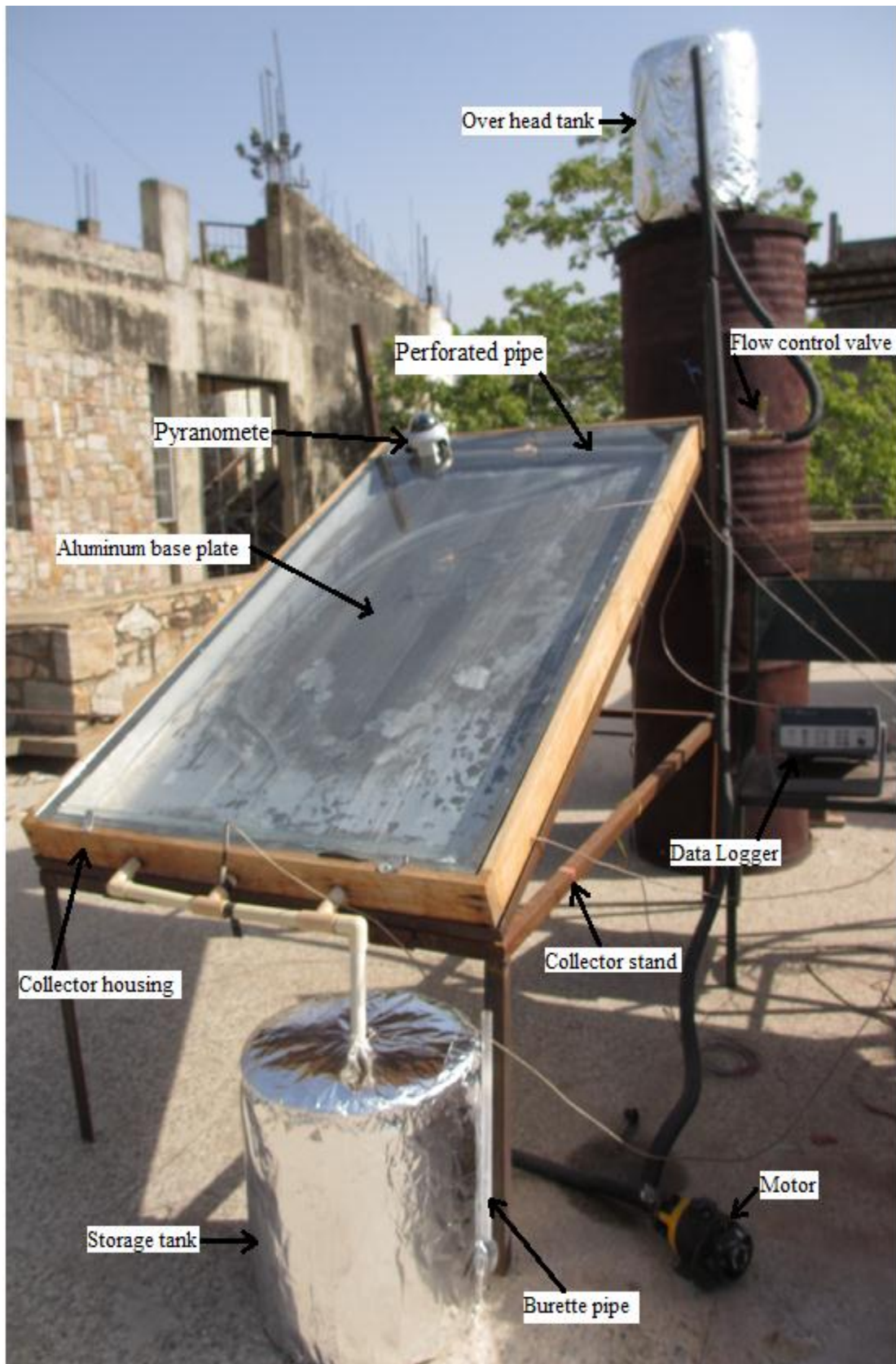
Fig. 4.13 Experimental Setup-II of DASC with aluminum base plate
