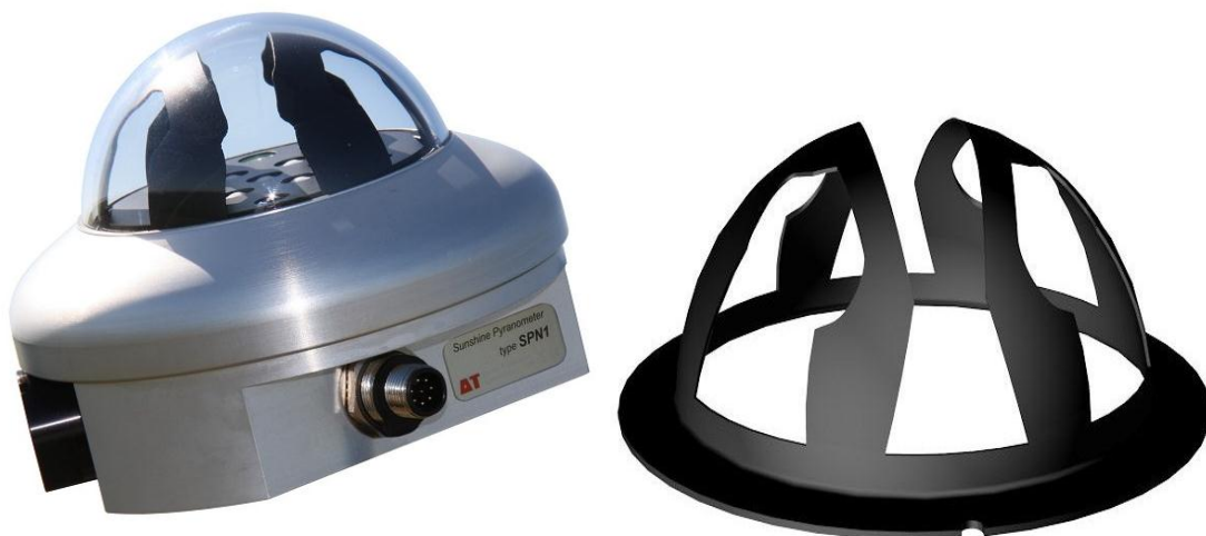
Fig. 4.18 Sunshine pyranometer (SPN1 type) and computer generated shadow mask
