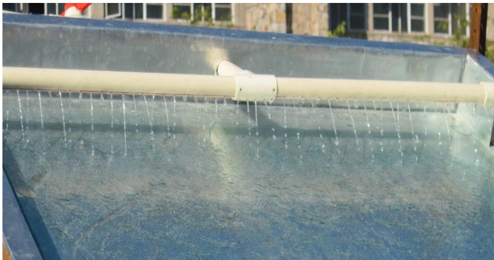
Fig. 4.5 Perforated pipe method for film formation
