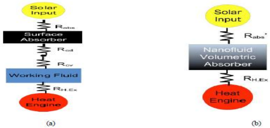
Fig. 1.3 a: Conventional collector b: Direct absorption solar collector
