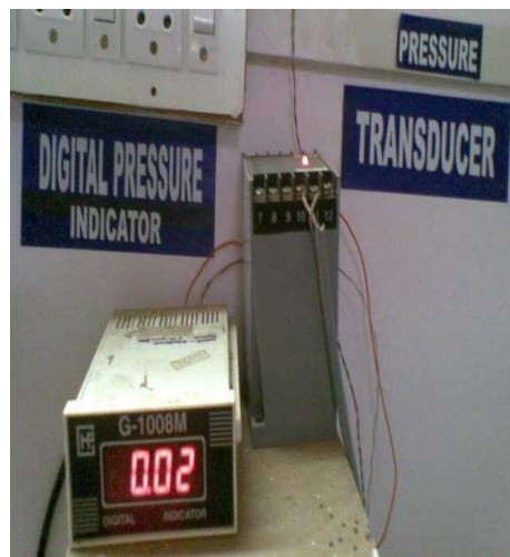
Figure 3.10. Photograph of pressure sensor and digital pressure indicator.
