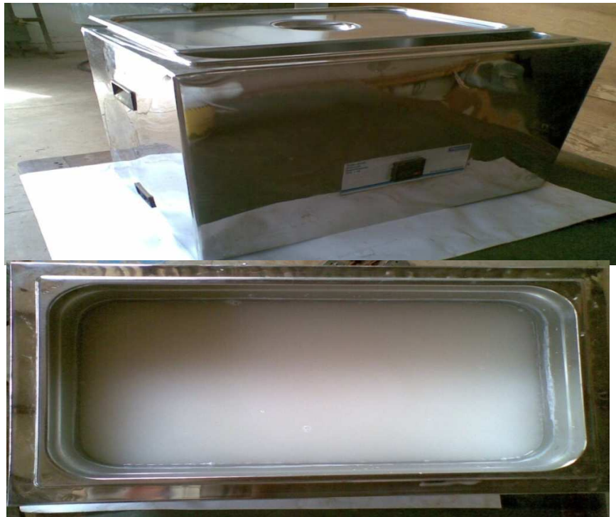
Figure 3.4. Photograph of Ultrasonic Vibration Mixer Machine Outer shell and prepared Al 2 O 3 -water nanofluids in UVM.
