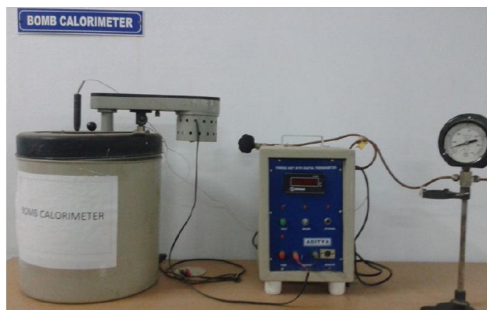
Figure 3:11 Bomb calorimeter for measuring calorific value of the fuel
