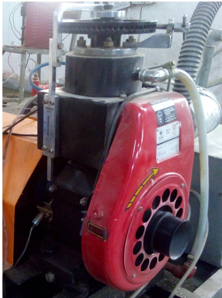
Figure 3:3 Single cylinder four stroke SI engine (Greaves make)
