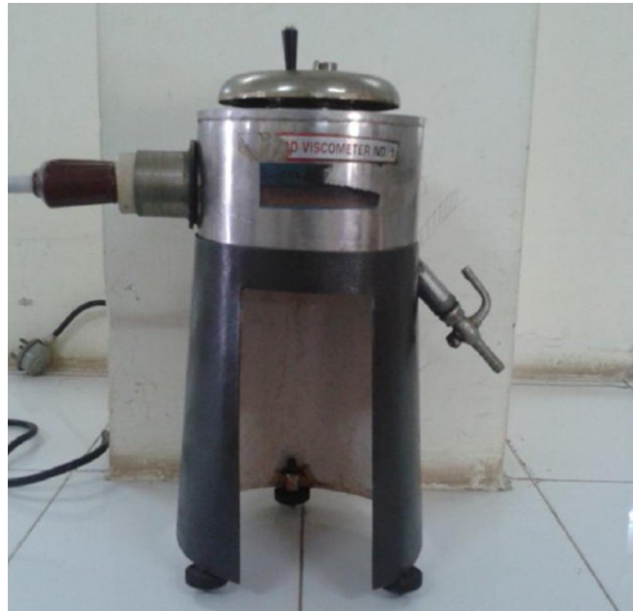
Figure 3:12 Redwood Viscometer for measuring viscosity of the fuel
