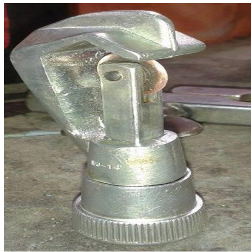
Fig.3.2 Pictorial view of Pipe cutter
