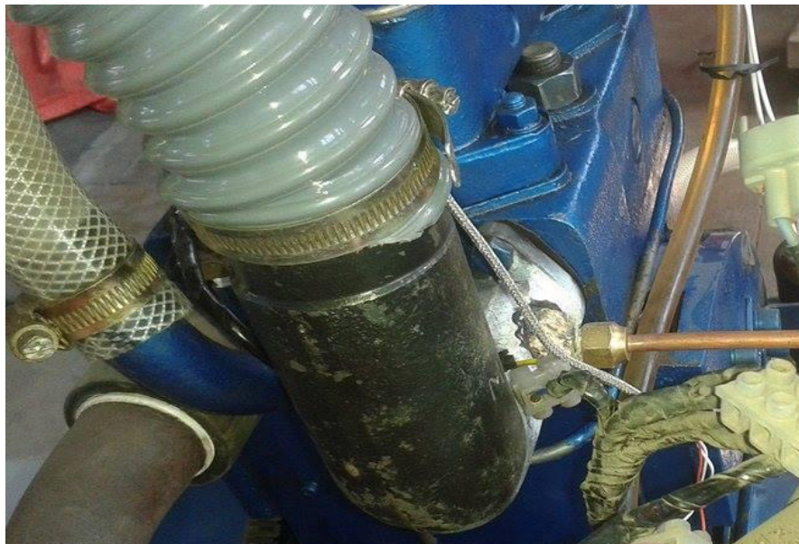
Fig.3.2 Pictorial view of Mixer (air inlet and Cu pipe for hydrogen enrichment)
