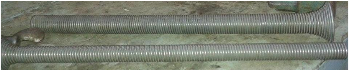
Fig.3.2 Pictorial view of Copper Pipe bender to assemble the set up
