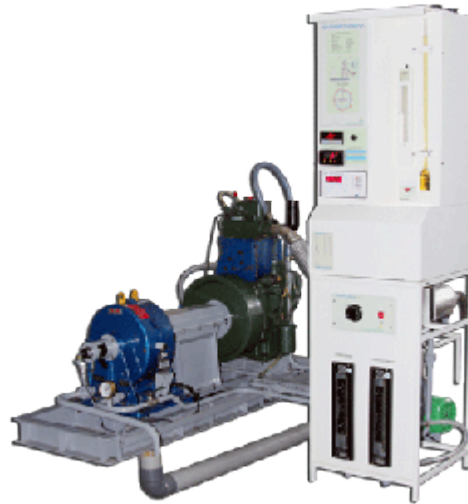
Figure 4.6: VCR experimental set up (Source:edutekindia.com)
