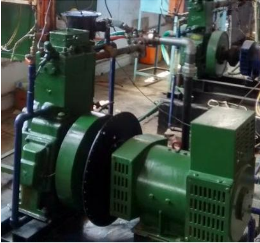
Figure 11 Kirloskar diesel engine coupled with electrical dynamometer
