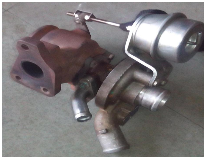
Figure 12 Turbocharger with Waste gate valve
