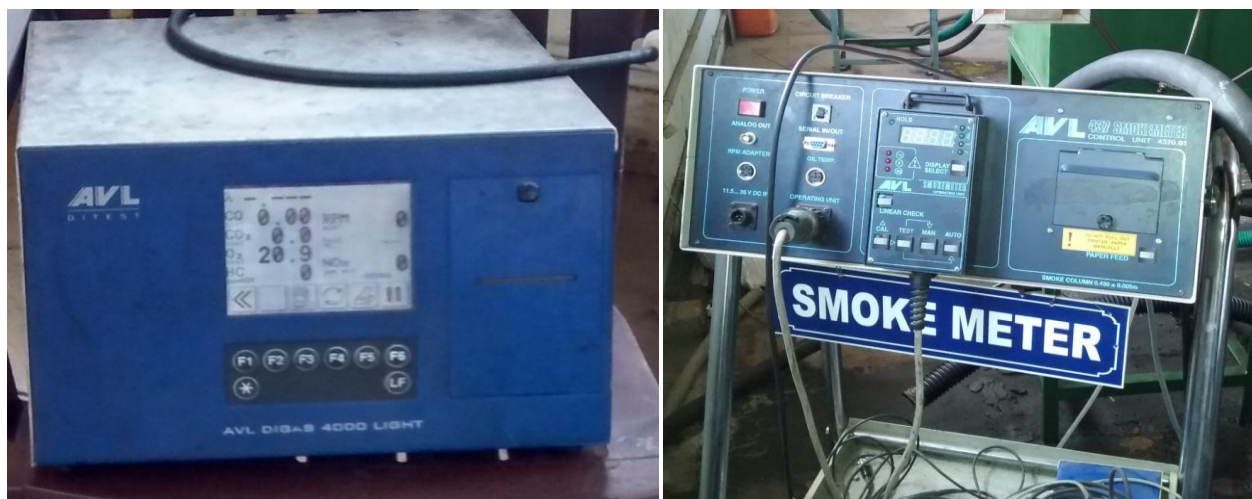
Figure 19 AVL DIGAS 4000 LIGHT (left) & AVL 437 SMOKEMETER (Right)
