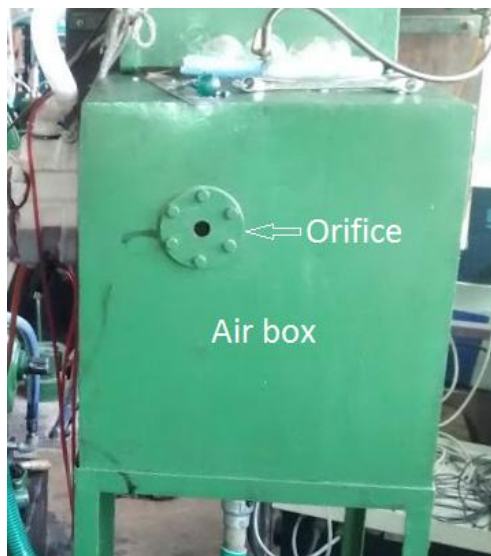
Figure 18 Air flow measuring system
