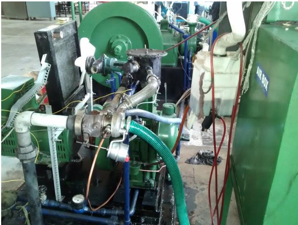
Figure 16 Experimental setup with turbocharger.
