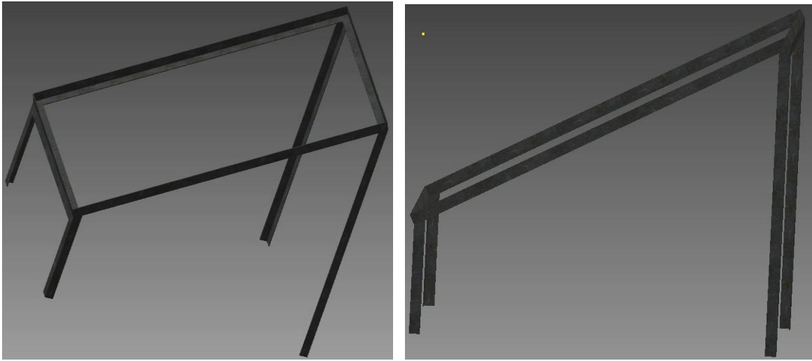
Figure 3.3: Stand of air heater
