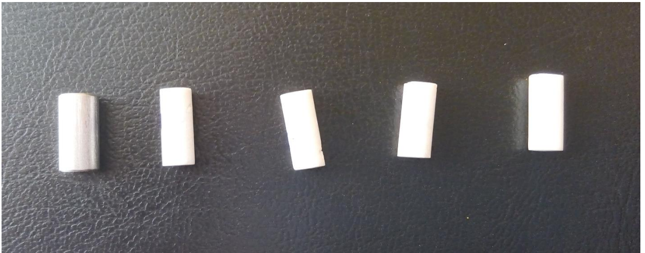
Fig. 3.3.1 Sample for wear and DMA test
