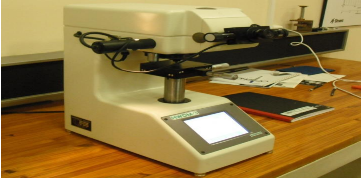
Fig 3.4.1 Apparatus used to determine the Vickers hardness number (VHN)
