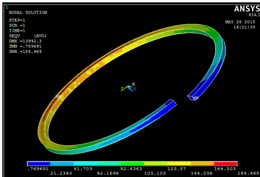
Figure 6.7 Stress developed in ring under uniformly distributed bending load
