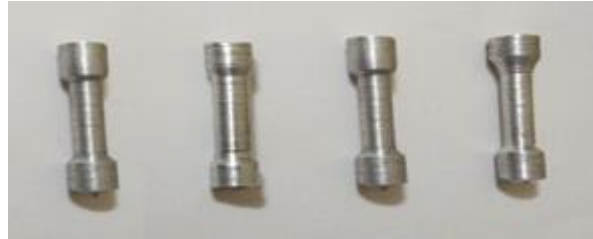
Figure3.6 Specimen for tensile test
