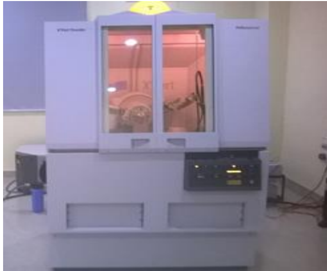
Figure 3.9 X-ray diffraction testing machine
