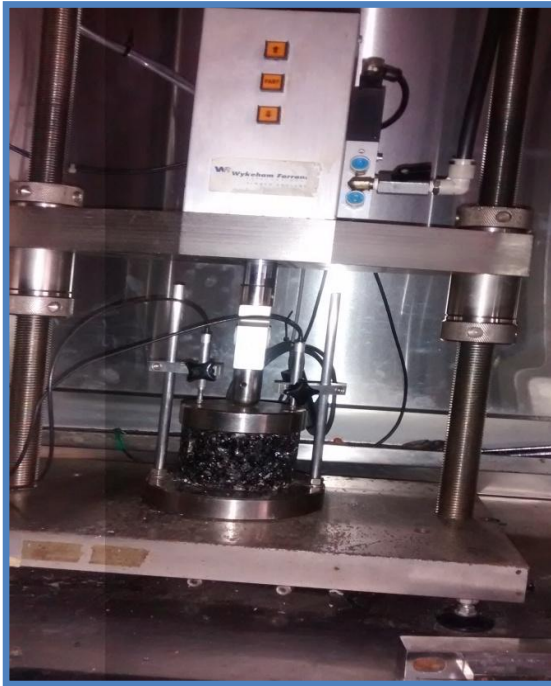
Fig. 3.14: Dynamic creep test set up
