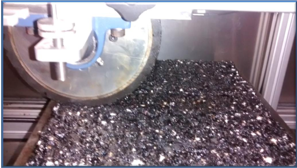
Fig. 3.18: Wheel Tracking Test in progress
