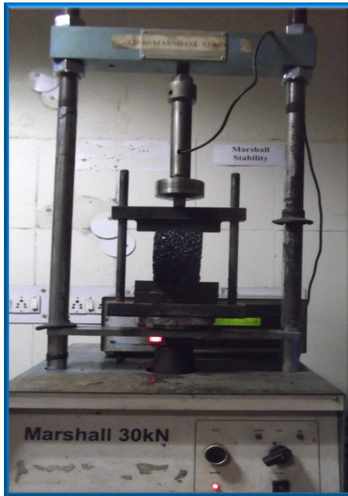
Fig. 3.11: Indirect Tensile Strength Test Set-up
