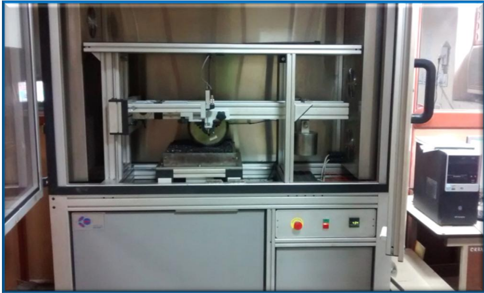
Fig. 3.19: Wheel Tracking Device Set-up
