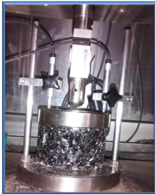
Fig. 3.15: Dynamic creep test specimen
