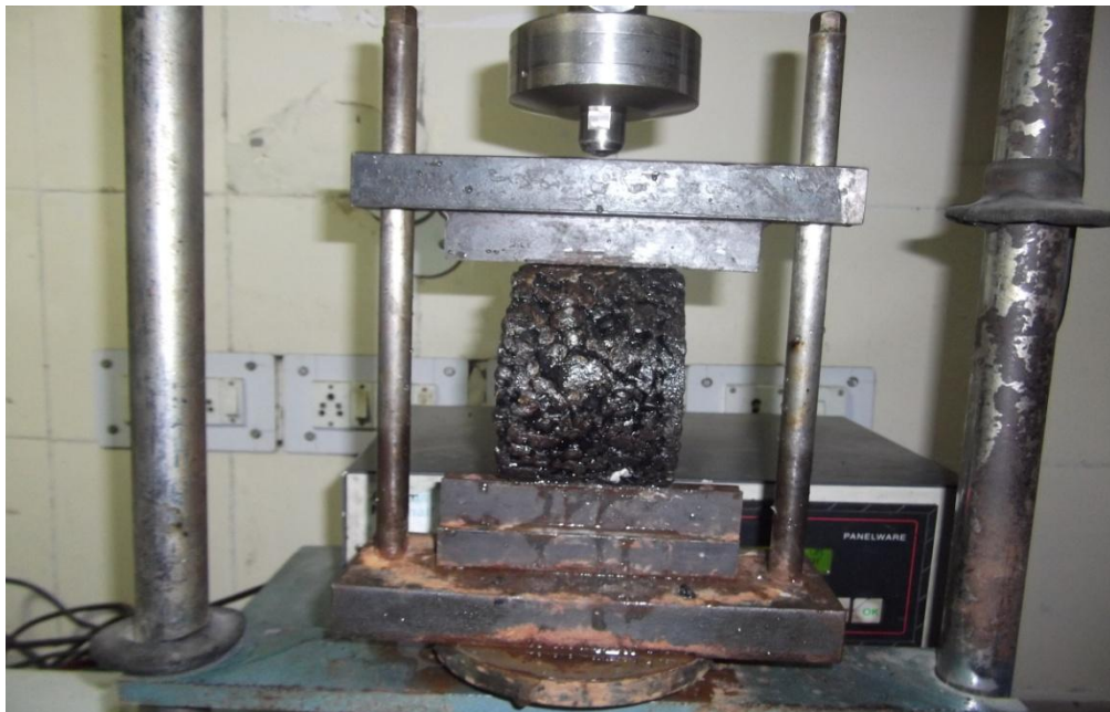
Fig. 4.17: Tensile Failure of Conditioned Specimen during ITS test
