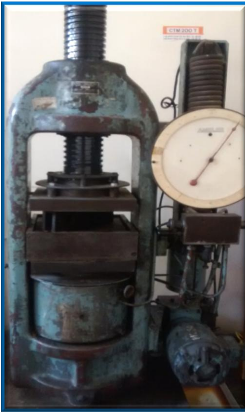
Fig. 3.16: Slab Compaction machine
