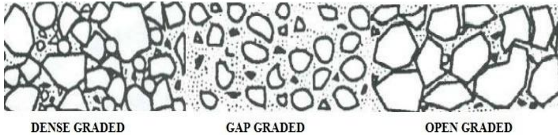
Fig. 2.1 Comparison of dense, gap and open gradation structure of HMA
