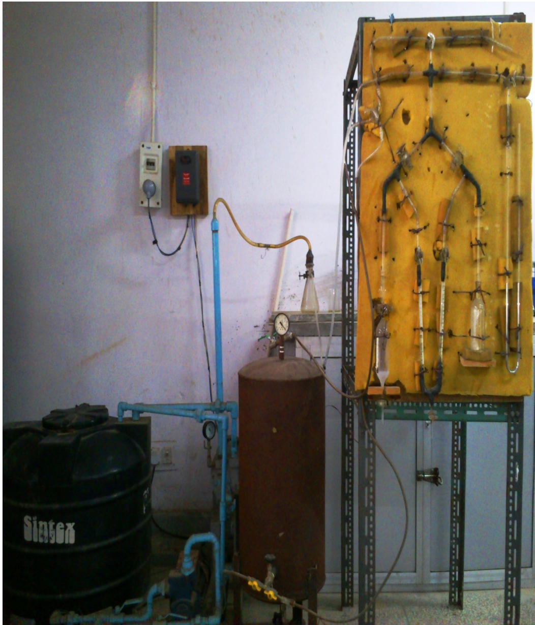
Figure 4C.1 Experimental set-up for measurement of surface coefficient
