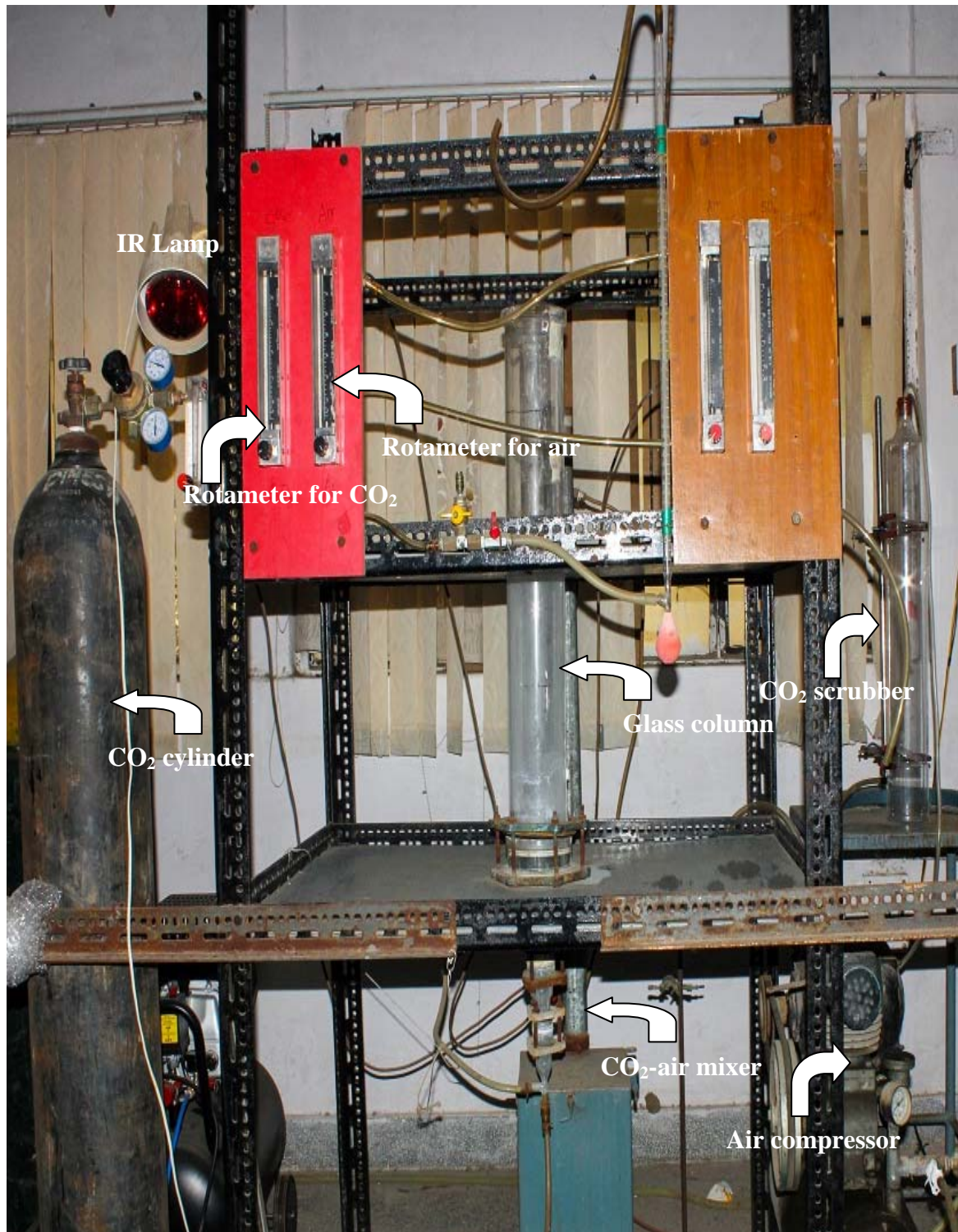
Figure 4.4 Experimental set-up used for gas-liquid-solid system
