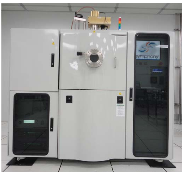
Figure 2.1: RF Sputtering setup
