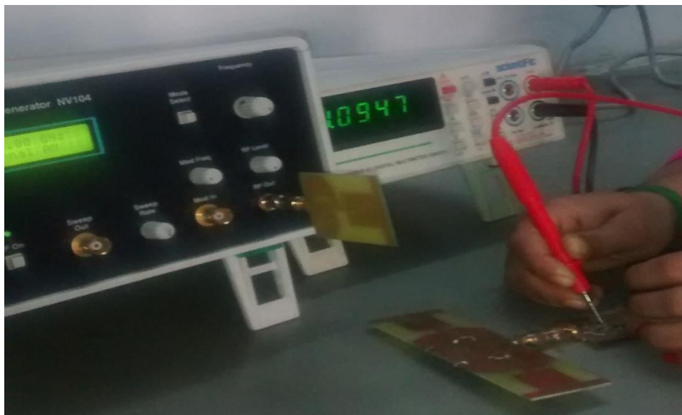
Fig. 5.11. RF-DC converter circuit with 2×1 array coplanar monopole antenna.
