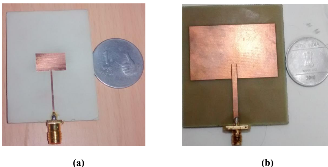
Fig. 3.7. (a) Fabricated antenna on substrate Rogers RO3210 ( \epsilon_{r2} = 10.2 ) (b) Fabricated antenna on substrate Rogers FR4 Epoxy ( \epsilon_{r2} = 4.4 )
