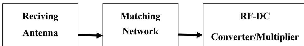
Fig. 5.1 General block diagram for the energy harvesting system.
