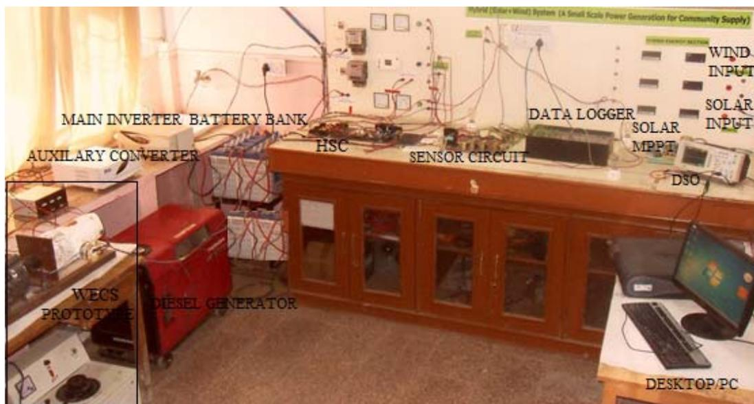
Figure 5.9 Overall view of stand-alone solar-wind-battery-diesel generator hybrid system
