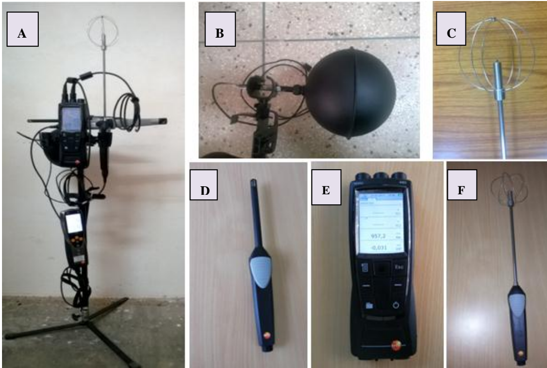
Figure 3-3 VAC 480 instrument for measuring thermal environmental variables
