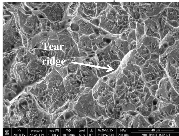
Figure 4.30e. SEM fractographs for 10 wt.-% of CaO particulate filled SiBr alloy composites after fracture test
