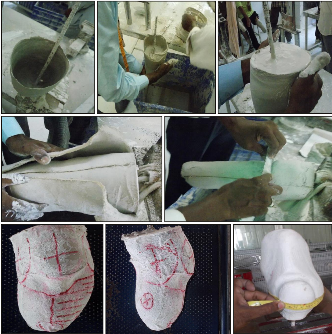
Figure-3.3: Manually modifications at patella tendon area in BMVSS, Jaipur, India
