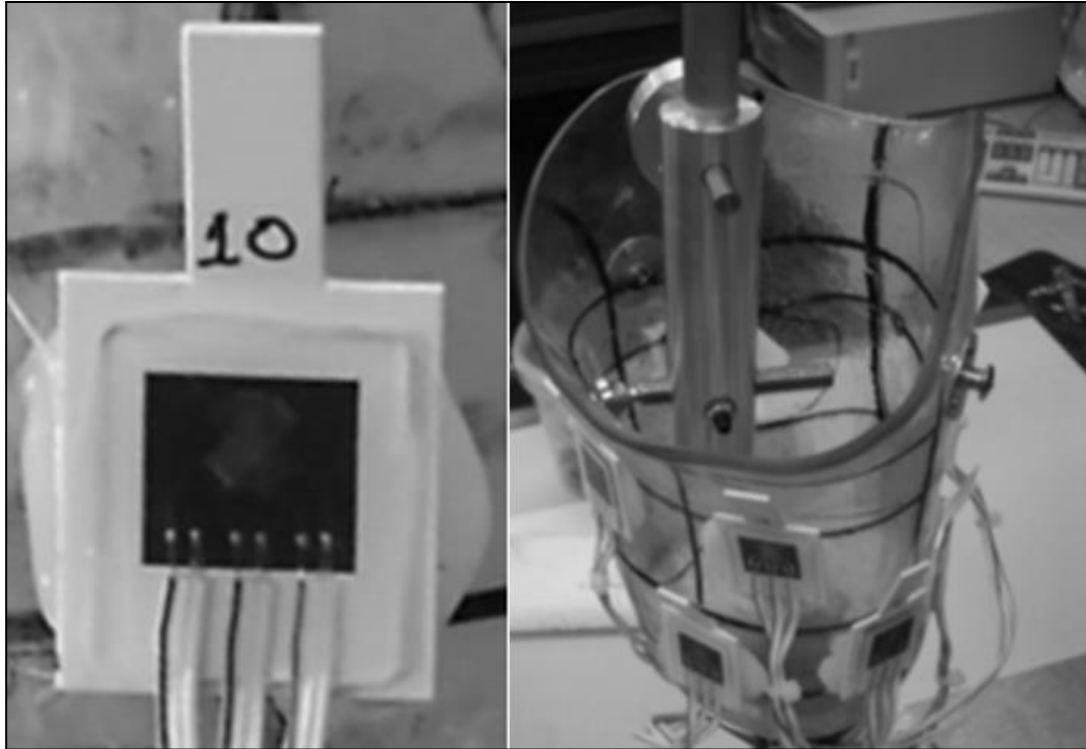
Figure 2.16: (a) Strain gauge based transducer (b) Pressure being applied on socket (Sewell, 2012)
