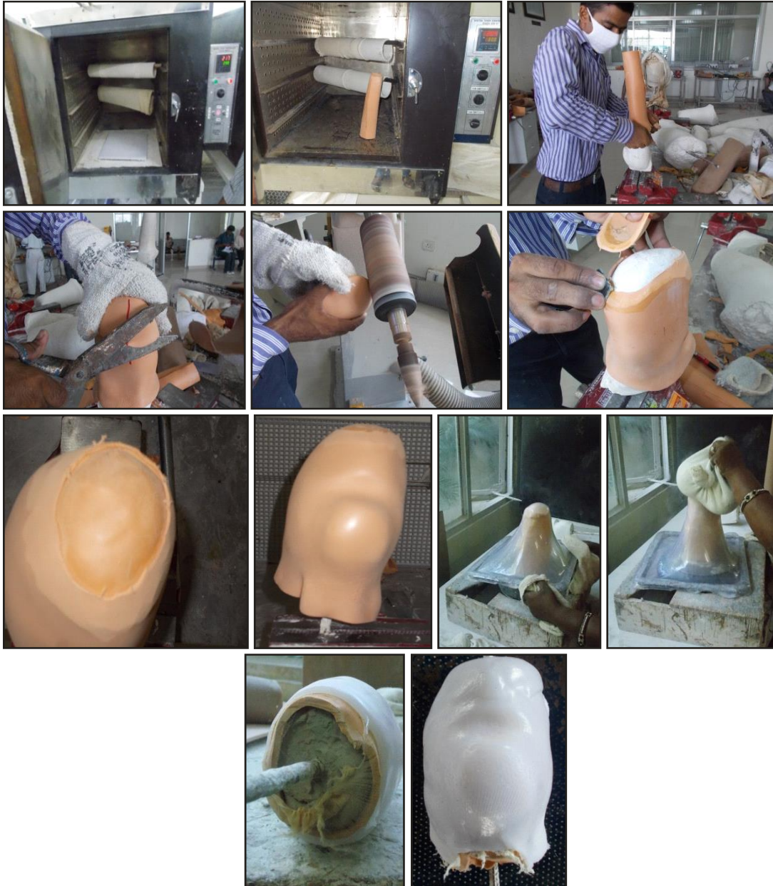
Figure-3.4: Fabrication and finishing of socket in BMVSS, Jaipur, India
