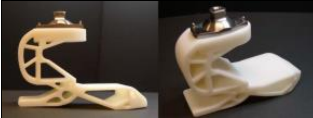
Figure-2.7: Optimized prosthetic feet using SLS technology (Nicholas 2009)
