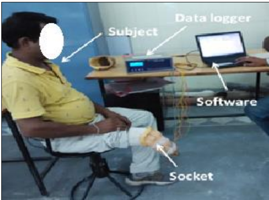
Figure-6.5: Photograph of instrumentation with patient
