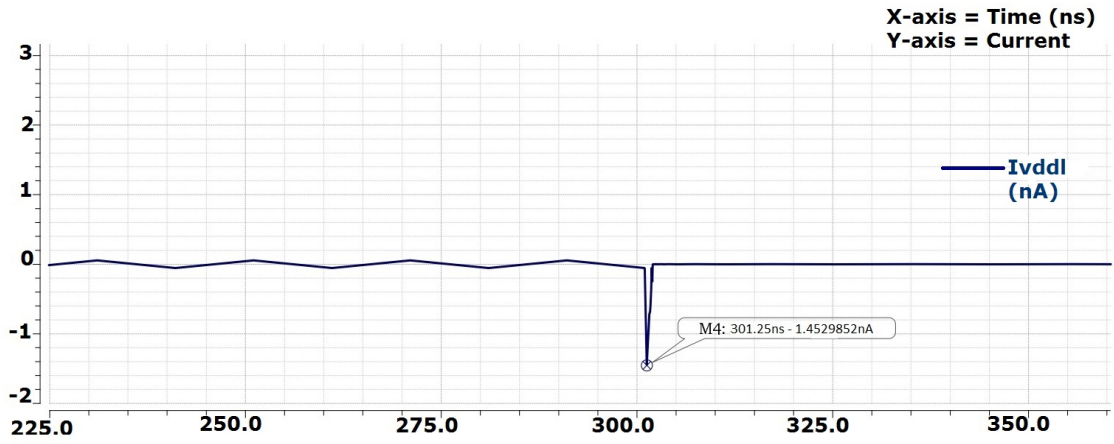
FIGURE 4.11: Static Current I_{vddl} for V_{ddl}=1.2\text{volt} and V_{ddh}=5\text{v}
