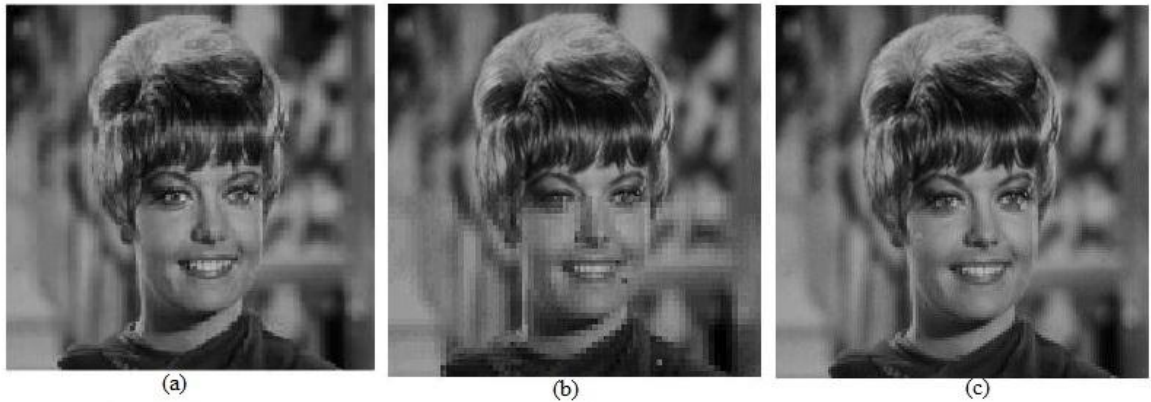
Figure-5.10: Recovered image Zelda at 50% tampering (a) host image, (b) reference scheme [4], (c) proposed scheme
