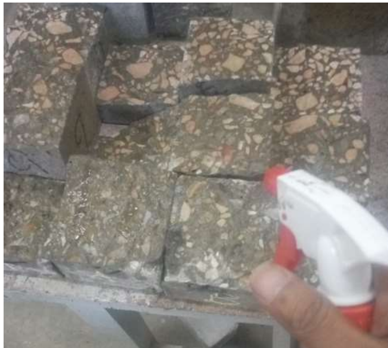
Figure 4.26: Spraying of 0.1N Silver Nitrate Solution on freshly split concrete specimens
