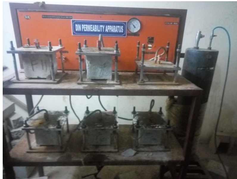
Figure 3.12: Water Penetration Apparatus as per DIN 1048
