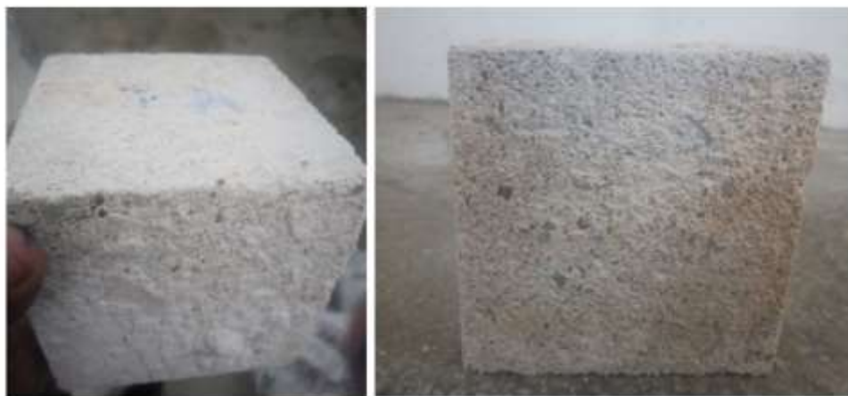
Figure 4.48: Control Concrete Specimens and Dholpur/quartz sandstone concrete samples after 180 days Sulphate Attack Test
