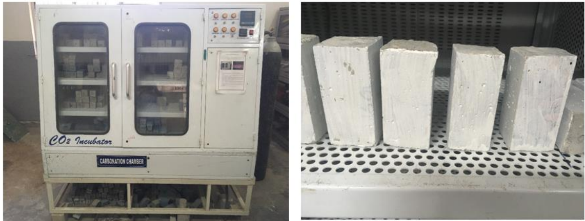
Fig 3.14: Carbonation chamber and Epoxy coated concrete samples
