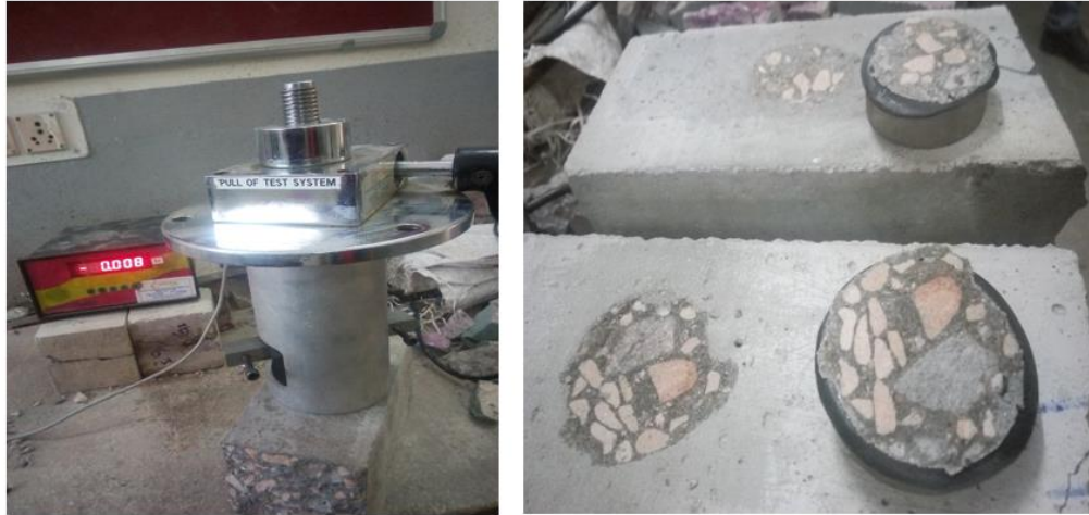
Figure 3.10: Procedure showing Pull-off strength testing
