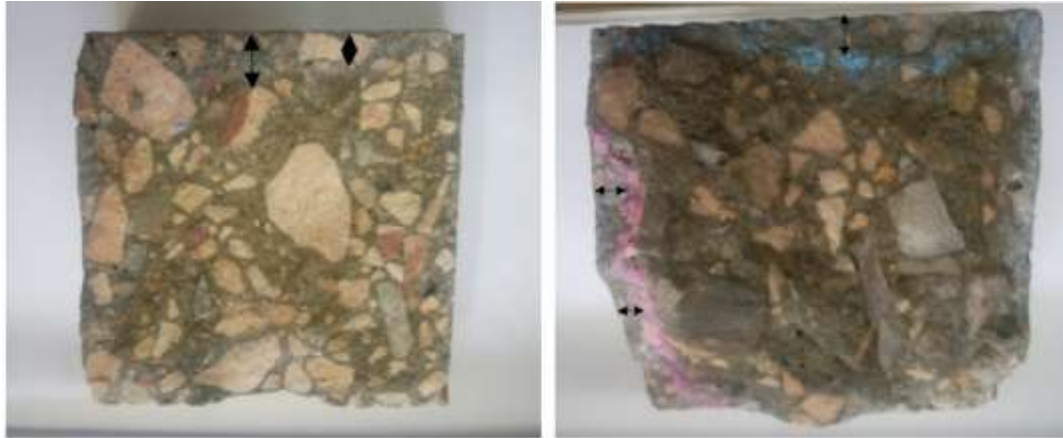
Figure 4.27: Freshly Split Concrete Specimens showing depth of Chloride Penetration after 28 days (Arrows indicate the depth of chloride penetration)
