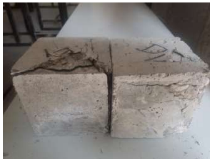
Fig 4.5. Broken samples after compressive strength testing
