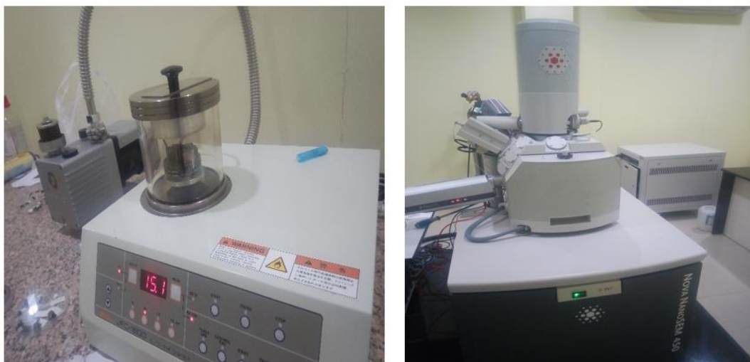
Figure 3.18: Coating device and FE-SEM machine with EDX attachment.
