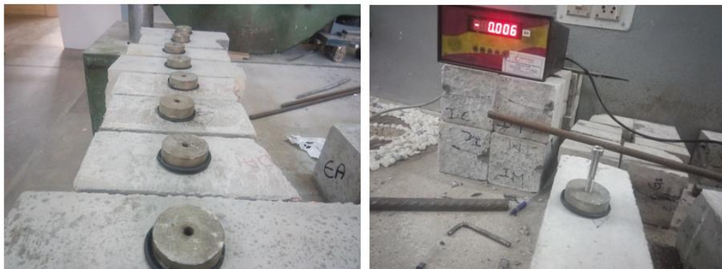
Figure 3.9: Pull-off set up on the concrete samples
