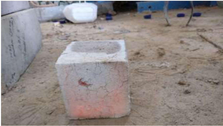
Figure 4.67: Concrete image after exposure to fire at 800°C.
