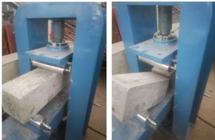
Fig 4.9: Arrangement and failure of test specimens under flexural loading
