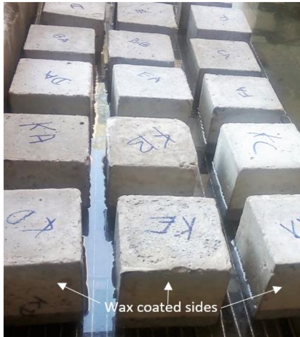
Figure 3.11: Test setup for sorptivity showing wax coated sides.
