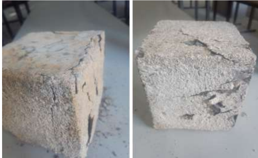
Figure 4.49: Sulphate attacked specimens after compressive strength testing at 90 and 180 days
