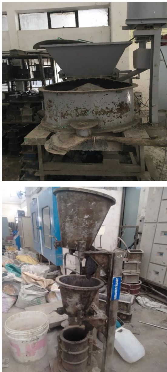
Figure 3.5: Concrete mixer and compaction factor apparatus
