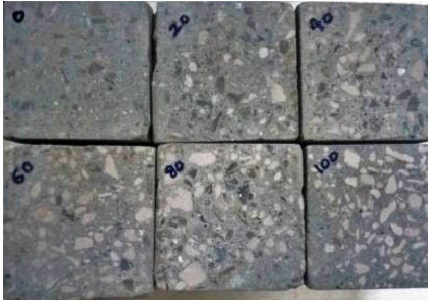
Figure 4.11: Abraded surface of concrete having quartz sandstone for various replacement levels
