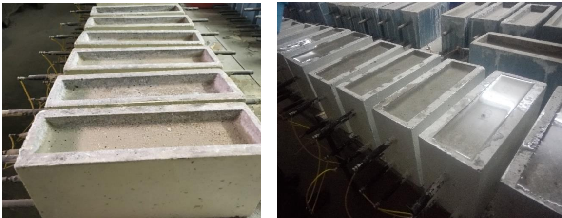
Figure 3.17: Epoxy coated specimens with 3% NaCl solution (drying and wetting cycle)
