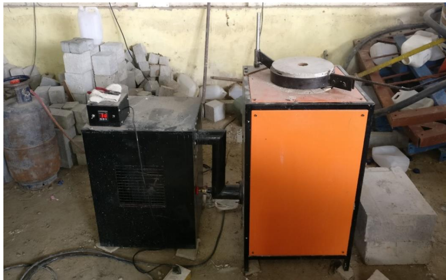
Figure 3.20: Equipment used to regulate fire in concrete samples.
