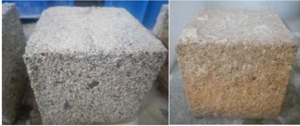
Figure 4.32: Acid attacked specimen at 90 days. Control concrete (left) and 100% (right) quartz sandstone.
