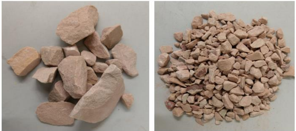
Fig 3.1: Dholpur aggregate (Quartz sandstone) aggregates of sizes 25 mm and 10mm.
