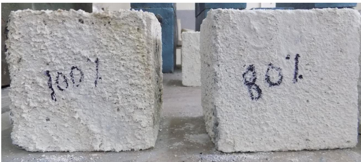
Fig. 8.1. Visual assessment of 180 days acid attack on FBA aggregate concrete
