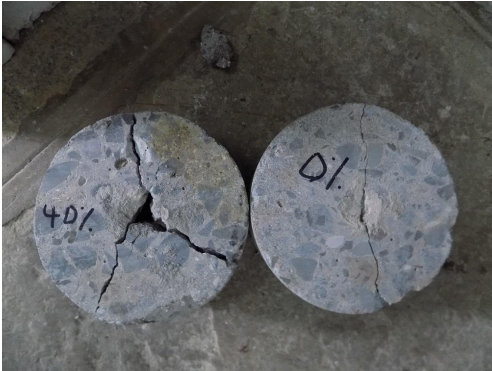
Fig. 9.1 Fracture pattern of concrete sample due to drop weight impact
