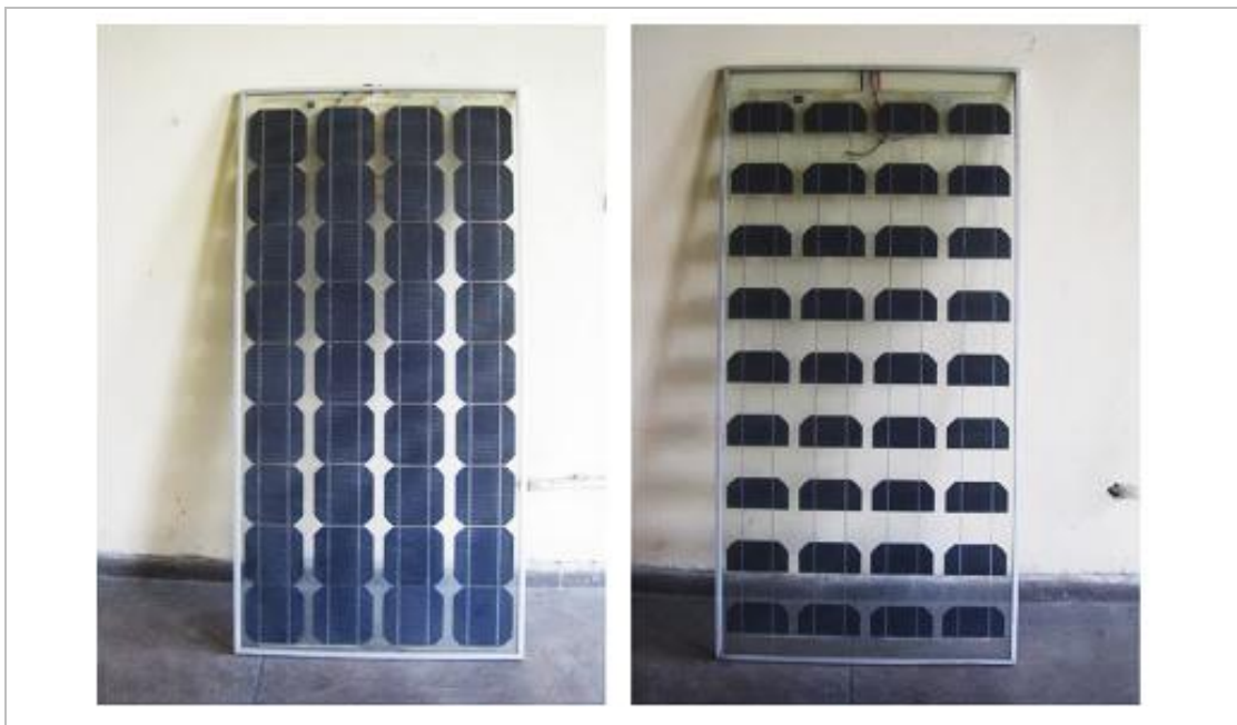
Figure 2-1: Crystalline Si photovoltaic modules with different packing factors [48]
