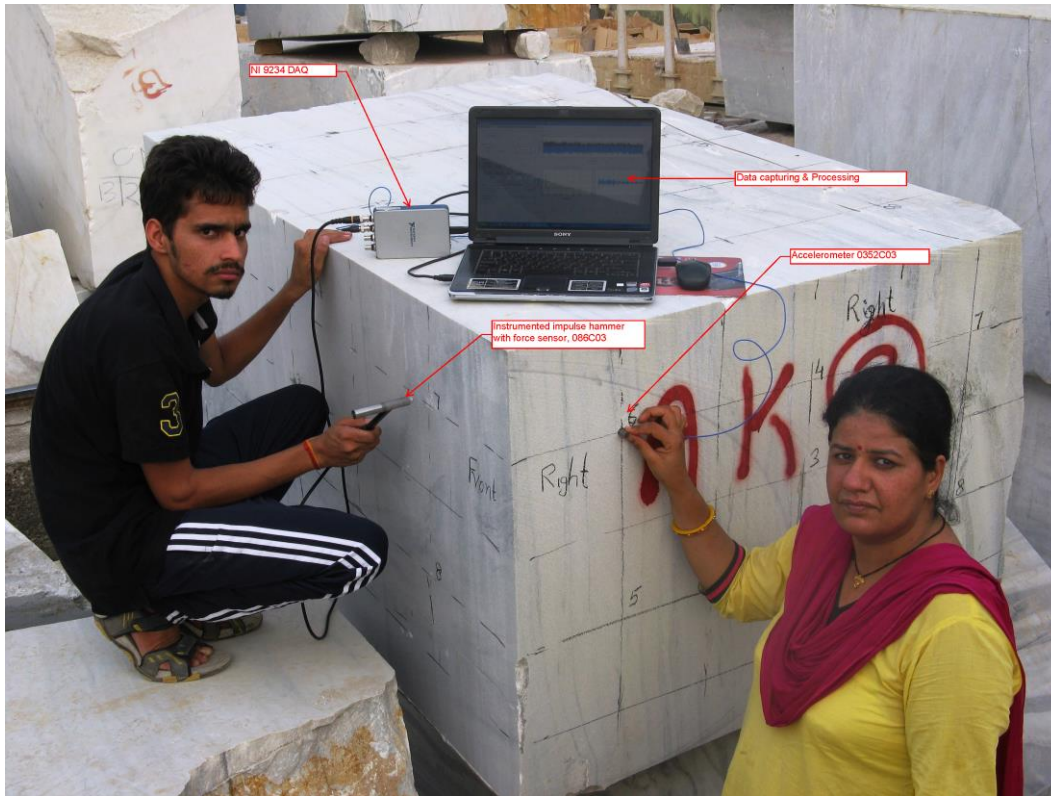
Figure 20: Photograph of data collection setup from a marble block in the field.
