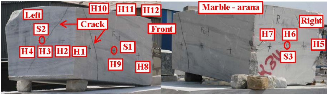
Figure 47: Face photos, hammer and accelerometer locations for stone block 2 (Arana marble).
