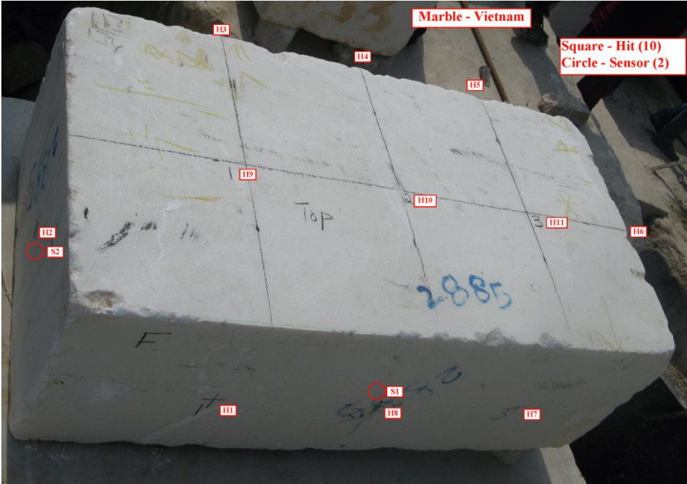
Figure 49: Face photos, hammer and accelerometer location for stone block 4 (Vietnam marble).
