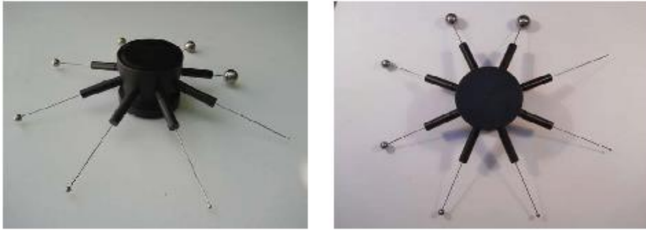
Figure 9: Impactor kit for the impact-echo method, containing impactors on springs connected to plastic cylinders and rubber couplings. The housing has a rubber ring resting against the surface. (Model Spider DOC-210N, taken from Germann Instruments A/S, www.germann.org )
