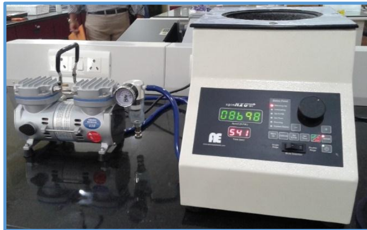
Figure 3.2: Spin coating unit used for present deposition.
