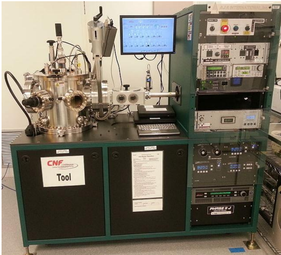
Figure 3.2. Magnetron co-sputtering setup (AJA International, Model- SHQ OR) used in present study at UGC-DAE CSR Indore.
